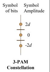
(b) Give a symbol of bits for each symbol amplitude on the 3-PAM constellation. Make sure that the bit encoding for adjacent symbols only differs by one bit (Gray coding). *6 points*.
