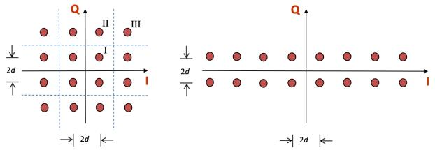
Energy in the pulse shape is 1. Symbol time  $T_{sym}$  is 1s. The constellation on the left includes the decision regions with boundaries shown by the in-phase (I) axis, quadrature (Q) axis and dashed lines.
