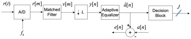
The adaptive FIR equalizer runs at the symbol rate and has N coefficients. We place the coefficients in a vector
