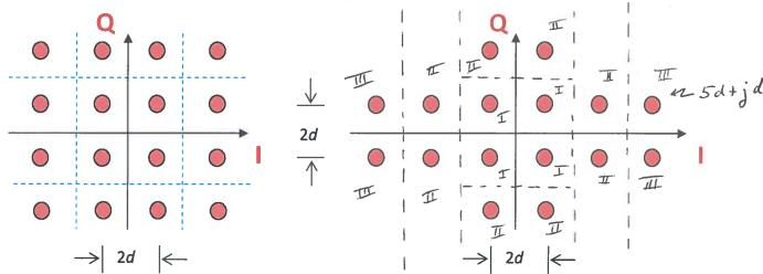
Energy in the pulse shape is 1. Symbol time  $T_{\text{sym}}$  is 1s. The constellation on the left includes the decision regions with boundaries shown by the in-phase (I) axis, quadrature (Q) axis and dashed lines.
