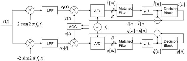
**System parameters**: *B* bits at A/D output, 2*d* constellation spacing,  $f_s$  sampling rate,  $f_{sym}$  symbol rate, *J* bits/symbol, *L* samples/symbol, and *M* constellation points (i.e.  $M = 2^J$ ). *B* is much greater than *J*.
