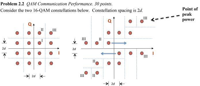
Energy in the pulse shape is 1. Symbol time  $T_{sym}$  is 1s. The constellation on the left includes the decision regions with boundaries shown by the in-phase (I) axis, quadrature (Q) axis and dashed lines.
