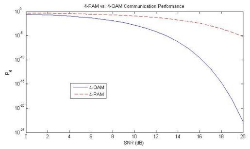
QAM performs much better than the PAM system due to the following reasons: first the noise variance in the PAM system is higher so we expect its error rate to be higher; on the other hand the PAM system is not fully utilizing the bandwidth as opposed to QAM.
