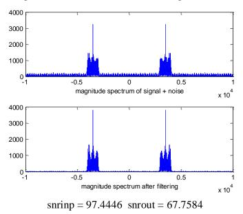
Some of the energy in the signal and interference resides outside the 3000-4000 Hz band. The bandpass filter passes a higher percentage of interference energy than signal energy.
