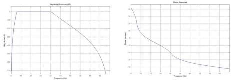
Chebyshev Type I: (Order 20) which has approximate linear phase over 15-30Hz.
