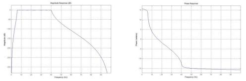
Chebyshev Type II (Order 20) which has approximate linear phase 15-30 Hz.
