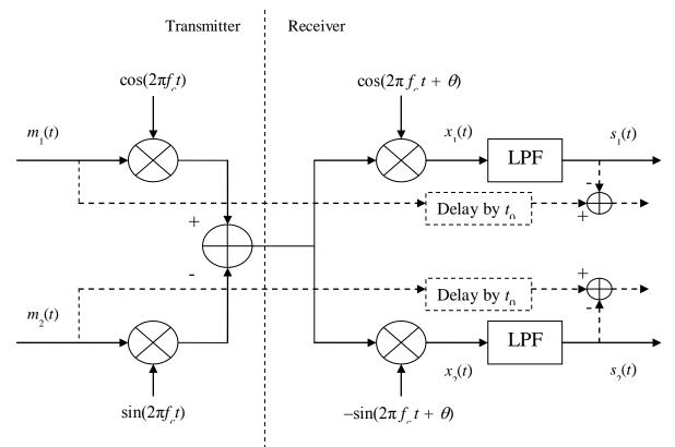
Note the negative sign on the sine carrier signal in the receiver to match the negated path for the sine carrier signal in the transmitter. Delay  $t_0$  matches the delay through the lowpass filter (LPF).
