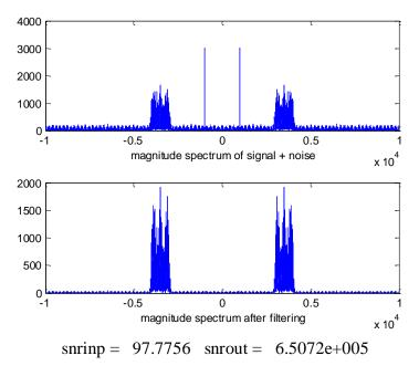
Solution for (b): Filter response for narrowband noise inside passband (SNR decreases):
