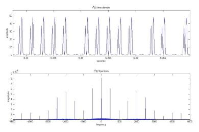
Other nonlinear functions will work. We could use exp(x) followed by a bandpass filter centered at  $2 f_0$  because  $exp(x) = 1 + x + (1/2!) x^2 + (1/3!) x^3 + ...$  from its series expansion.
