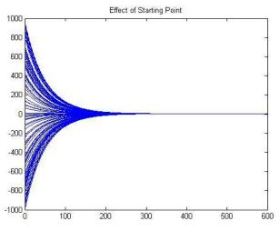
This plot shows with 100 different starting points ranging from -1000 to 1000, all of the curves converge to our desired value of x = 4.
