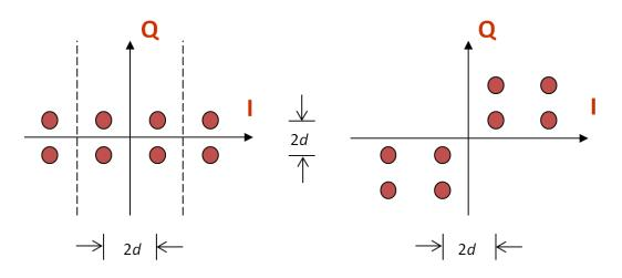
Energy in pulse shape is 1. Symbol time  $T_{sym}$  is 1s. The constellation on the left includes the decision regions with boundaries shown by the I axis, Q axis and dashed lines.
