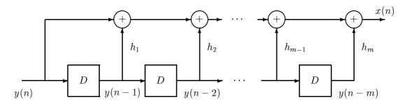
If y(n) is corrupted by channel errors, the scrambler output will also contain errors. If h(D) has K nonzero coefficients, a single isolated error in y(n) will cause K output errors as it propagates by the nonzero coefficients. Therefore, a connection polynomial with the least number of nonzero coefficients should be chosen.
