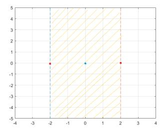
Pole-zero plot for the Laplace transform. ROC is shaded in yellow. The red dots denote the poles at s = 2 and s = -2. There are no zeroes. The blue dot denotes the origin.
