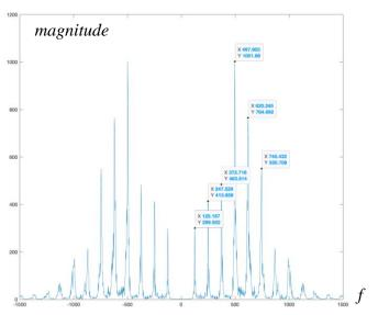
and negative frequencies needed to synthesize the vowel sound through trial-and-error by changing the value of Nkeep. The script keeps the Nkeep strongest frequency components.
