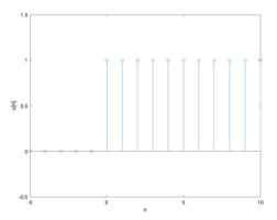
**Solution for (b):** Since the unit step signal is 0 for n < 0, x[n] for n < 0 is equal to 0. For  $n \ge 0$ ,
