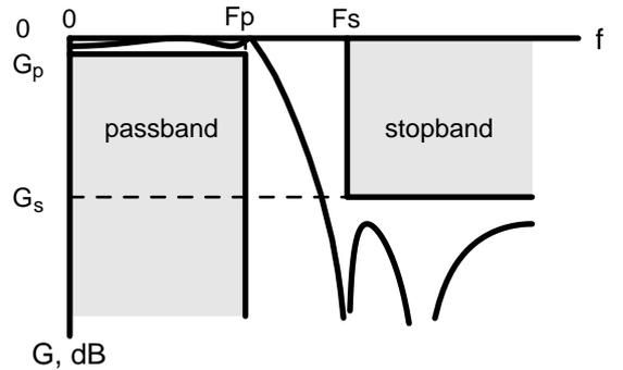
Fig. 6. Gain limit specification.
