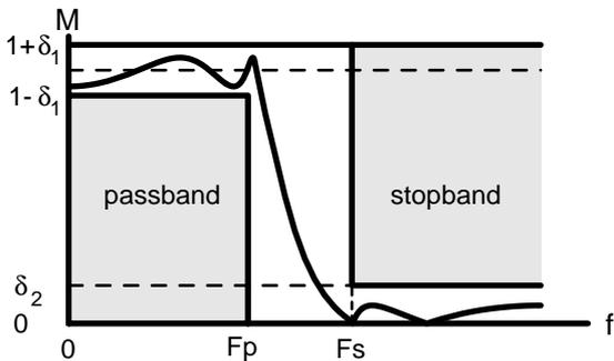
Fig. 4. Magnitude ripple specifications.
