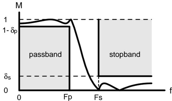
Fig. 3. Magnitude - tolerance specification.
