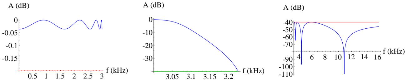
Fig. 17. Design 2:  $D = \{n_{min}, F_s/F_p, \epsilon < \epsilon_{max}, F_p\}$  for  $S_A = \{F_p = 3\text{kHz}, F_s = 3.225\text{kHz}, A_p = 0.2\text{dB}, A_s = 40\text{dB}\}$
