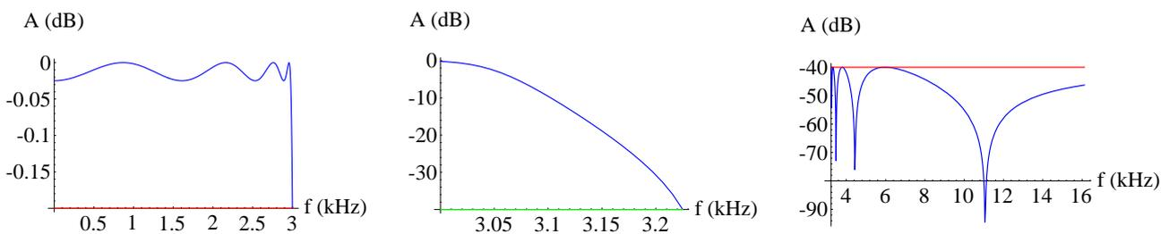
Fig. 21. Design 4b:  $D = \{n_{min}, a_{max}, \epsilon_{min}, F_s/a_s\}$  for  $S_A = \{F_p = 3\text{kHz}, F_s = 3.225\text{kHz}, A_p = 0.2\text{dB}, A_s = 40\text{dB}\}$
