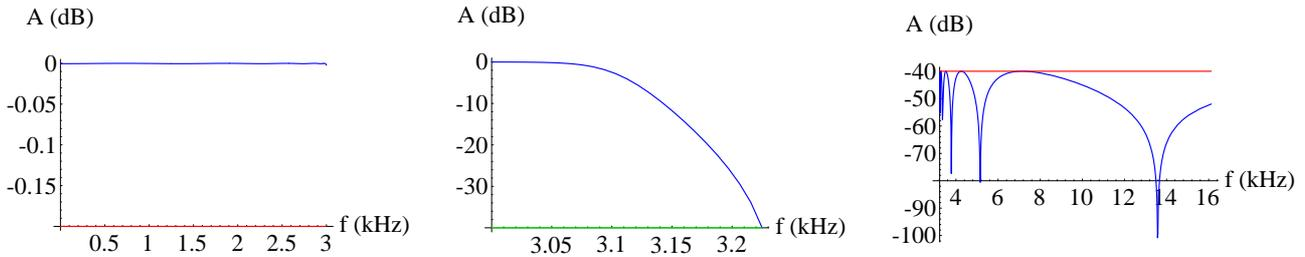
Fig. 23. Design 5a:  $D = \{n > n_{min}, a > F_s/F_p, \epsilon \ll \epsilon_{max}, F_s/a\}$  for  $S_A = \{F_p = 3\text{kHz}, F_s = 3.225\text{kHz}, A_p = 0.2\text{dB}, A_s = 40\text{dB}\}$
