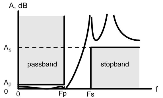
Fig. 5. Attenuation limit specification.
