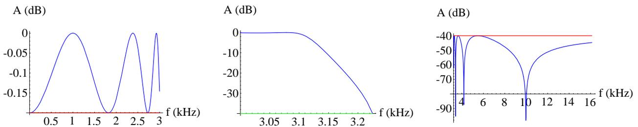
Fig. 19. Design 3b:  $D = \{n_{min}, a_{min}, \epsilon_{max}, F_s/a_s\}$  for  $S_A = \{F_p = 3\text{kHz}, F_s = 3.225\text{kHz}, A_p = 0.2\text{dB}, A_s = 40\text{dB}\}$
