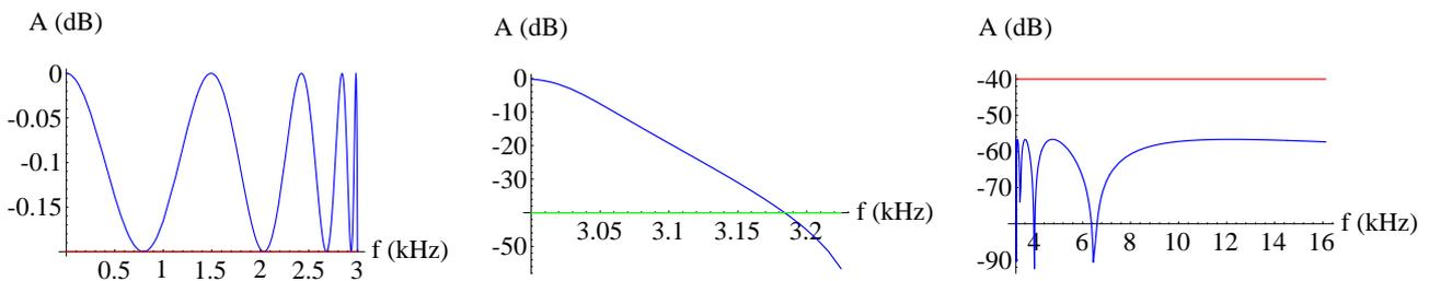
Fig. 26. Design 1:  $D = \{n_{min} + 1, F_s/F_p, \epsilon_{max}, F_p\}$  for  $S_A = \{F_p = 3\text{kHz}, F_s = 3.225\text{kHz}, A_p = 0.2\text{dB}, A_s = 40\text{dB}\}$
