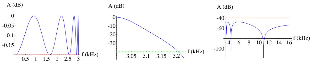
Fig. 16. Design 1:  $D = \{n_{min}, F_s/F_p, \epsilon_{max}, F_p\}$  for  $S_A = \{F_p = 3\text{kHz}, F_s = 3.225\text{kHz}, a_p = 0.2\text{dB}, a_s = 40\text{dB}\}$
