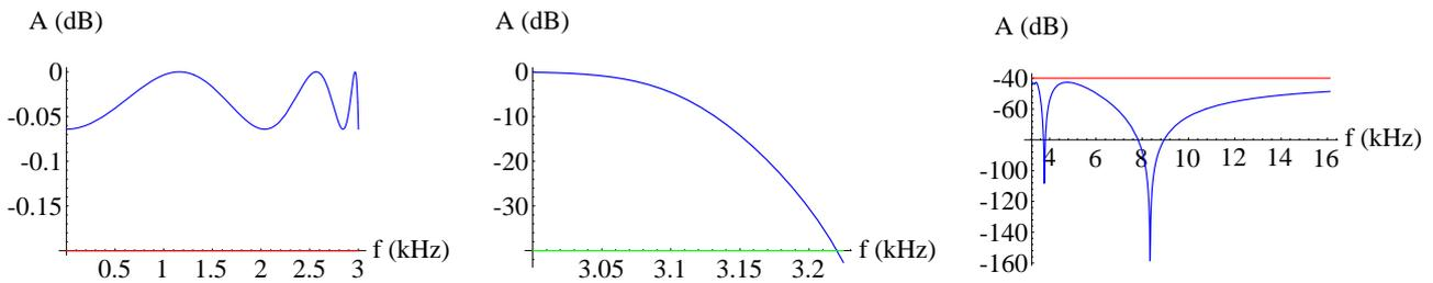
Fig. 25. Design  $D = \{2 \times 5, F_s/F_p, \epsilon_{max}, F_p\}$  for  $S_A = \{F_p = 3\text{kHz}, F_s = 3.225\text{kHz}, A_p = 0.2\text{dB}, A_s = 40\text{dB}\}$
