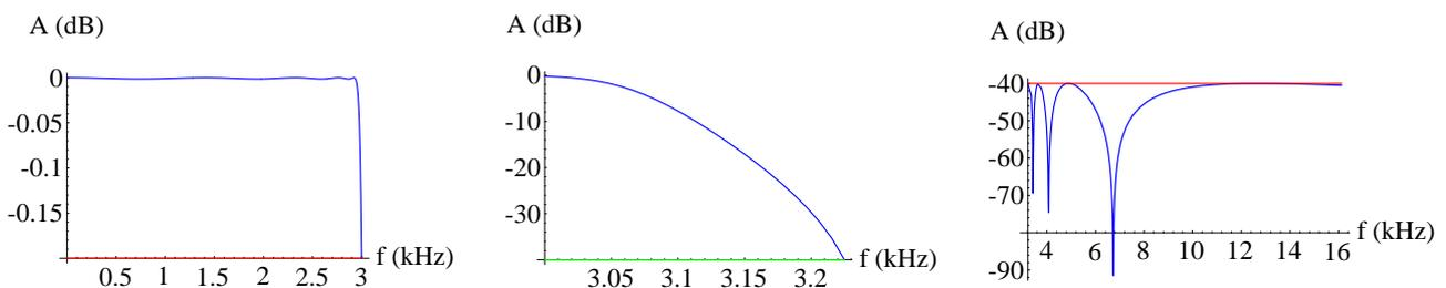
Fig. 31. Design 4b:  $D = \{n_{min} + 1, a_{max}, \epsilon_{min}, F_s/a\}$  for  $S_A = \{F_p = 3\text{kHz}, F_s = 3.225\text{kHz}, A_p = 0.2\text{dB}, A_s = 40\text{dB}\}$
