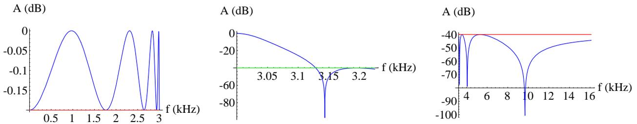
Fig. 18. Design 3a:  $D = \{n_{min}, a_{min}, \epsilon_{max}, F_p\}$  for  $S_A = \{F_p = 3\text{kHz}, F_s = 3.225\text{kHz}, A_p = 0.2\text{dB}, A_s = 40\text{dB}\}$
