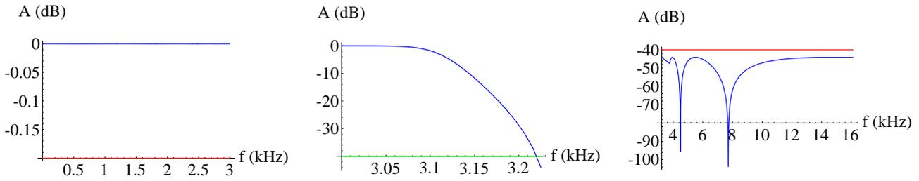
Fig. 22. Design 5:  $D = \{n > n_{min}, F_s/F_p, \epsilon \ll \epsilon_{max}, F_p\}$  for  $S_A = \{F_p = 3\text{kHz}, F_s = 3.225\text{kHz}, A_p = 0.2\text{dB}, A_s = 40\text{dB}\}$
