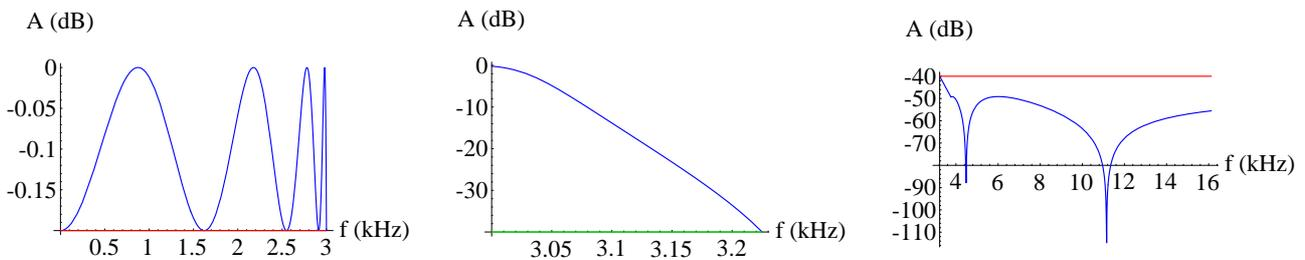
Fig. 20. Design 4a:  $D = \{n_{min}, a_{max}, \epsilon_{max}, F_p\}$  for  $S_A = \{F_p = 3\text{kHz}, F_s = 3.225\text{kHz}, A_p = 0.2\text{dB}, A_s = 40\text{dB}\}$
