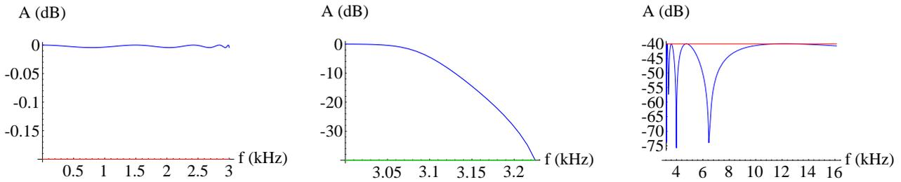
Fig. 27. Design 2:  $D = \{n_{min} + 1, F_s/F_p, \epsilon < \epsilon_{max}, F_p\}$  for  $S_A = \{F_p = 3\text{kHz}, F_s = 3.225\text{kHz}, A_p = 0.2\text{dB}, A_s = 40\text{dB}\}$
