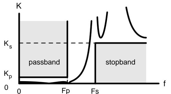
Fig. 7. Characteristic function limit specification.
