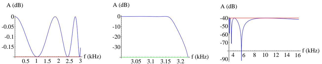
Fig. 29. Design 3b:  $D = \{n_{min} + 1, a_{min}, \epsilon_{max}, F_s/a\}$  for  $S_A = \{F_p = 3\text{kHz}, F_s = 3.225\text{kHz}, A_p = 0.2\text{dB}, A_s = 40\text{dB}\}$
