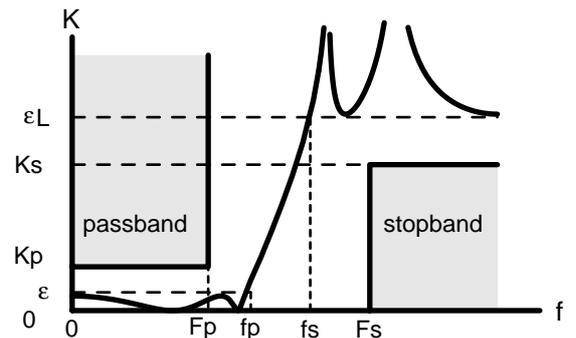
Fig. 8. Characteristic function.
