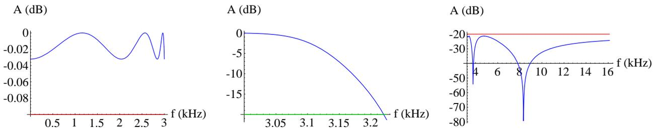
Fig. 24. Design 5:  $D = \{n > n_{min}, F_s/F_p, \epsilon_{max}, F_p\}$  for  $S_A = \{F_p = 3\text{kHz}, F_s = 3.225\text{kHz}, A_p = 0.1\text{dB}, A_s = 20\text{dB}\}$
