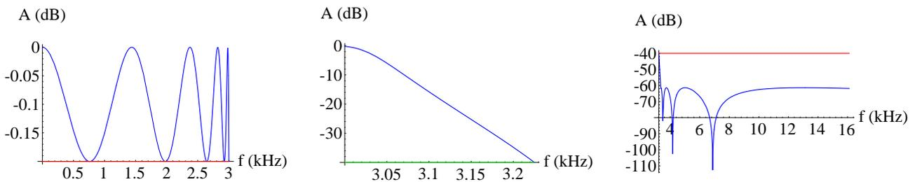
Fig. 30. Design 4a:  $D = \{n_{min} + 1, a_{max}, \epsilon_{max}, F_p\}$  for  $S_A = \{F_p = 3\text{kHz}, F_s = 3.225\text{kHz}, A_p = 0.2\text{dB}, A_s = 40\text{dB}\}$
