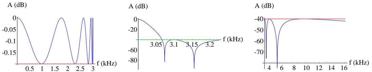
Fig. 28. Design 3a:  $D = \{n_{min} + 1, a_{min}, \epsilon_{max}, F_p\}$  for  $S_A = \{F_p = 3\text{kHz}, F_s = 3.225\text{kHz}, A_p = 0.2\text{dB}, A_s = 40\text{dB}\}$
