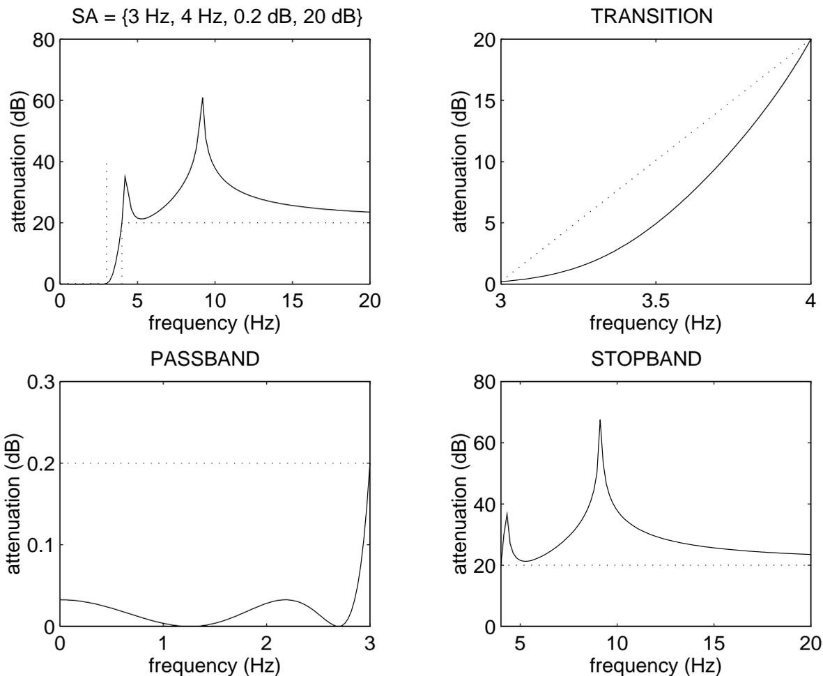
Fig. 1. Attenuation characteristic of an EMQF filter for  $S_A = \{3 \text{ Hz}, 4 \text{ Hz}, 0.2 \text{ dB}, 20 \text{ dB}\}$ .
