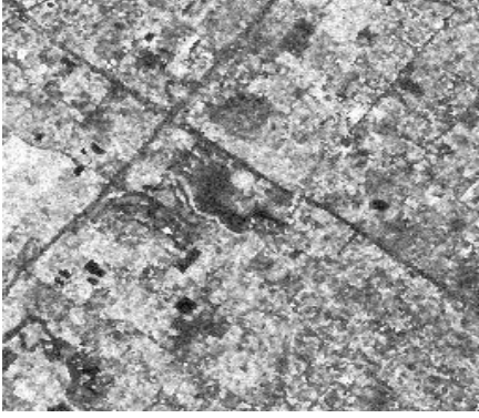
Figure 2: SAR image in Fig. 1 with additive white noise (PSNR is 23.1 dB with respect to Fig. 1).
