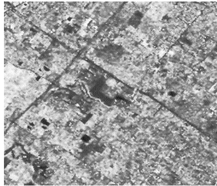
Figure 4: SAR image in Fig. 1 with additive highpass noise (PSNR is 23.1 dB with respect to Fig. 1).
