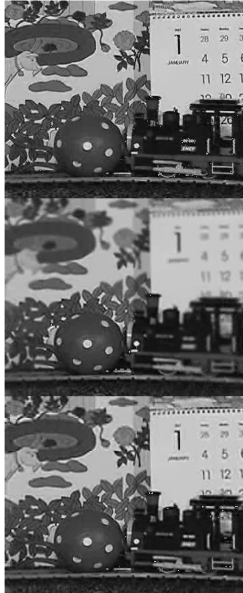
Fig. 5. Tenth reconstruction frame at the output of the H.263 decoder. Top to bottom: no foveation (uniform resolution) at the encoder, spatial domain foveation and DCT domain foveation. Fixation point is the center of the ball.
