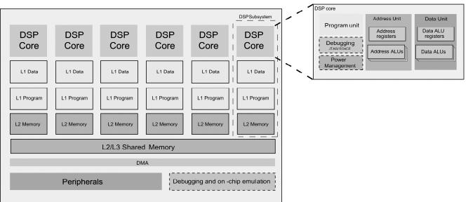
Fig.3. Typical multi-core DSP platform.
