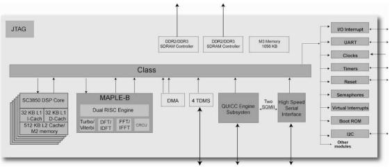
Fig.6. Freescale 8156 multi-core DSP processor.
