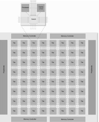
Fig. 9. Tilera TILE64 multi-core DSP processor.
