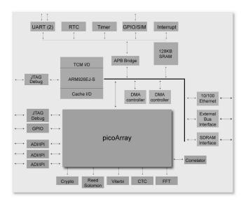
Fig.7. picoChip PC205 multi-core DSP processor.
