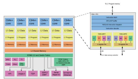
Fig.5. Texas Instruments TNETV3020 multi-core DSP processor.
