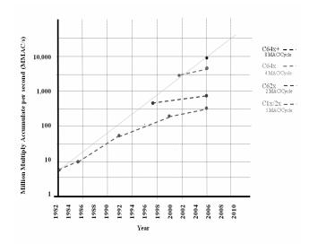
Fig. 2. Four generations of DSPs show how multi-processing has more effect on performance than clock rate. The dotted lines correspond to the increase in performance due to clock increases within an architecture. The solid line shows the increase due to both the clock increase and the parallel processing.
