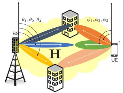
Figure 8: Angles of departure and arrival and associated channel gains
