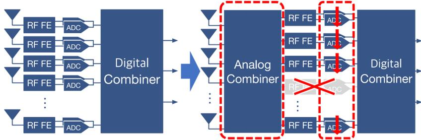
Figure 1: Power-efficient massive MIMO receiver architecture.
