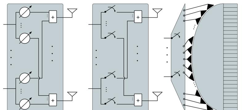
Figure 11: Phase shifter, switch and discrete lens array based architectures
