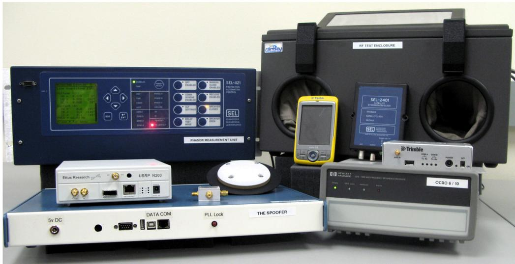
Figure 1.1: The University of Texas at Austin Radionavigation Laboratory spoofing test and development platforms. Shown here are a synchrophasor measurement unit (upper left), radio-frequency test chamber (upper right), civil GPS spoofer (lower left), cell phone base station oscillator (lower right), and several antennas and commercial receivers.
