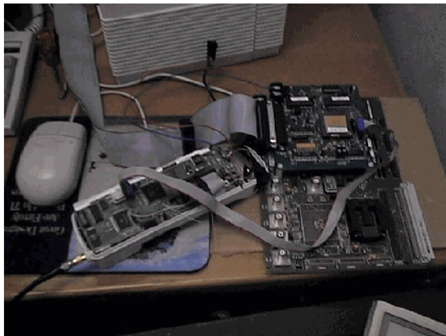
Figure A.7: A handset and emulator board
