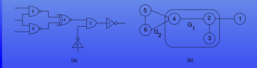
Figure 6: (a) A circuit to be partitioned (b) Its corresponding graph
