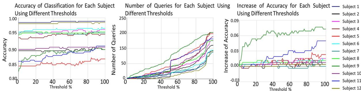
Fig. 7. Simulation results after performing Uncertainty Sampling. Accuracy, number of queries, and increase in accuracy for each subject is shown based on the uncertainty threshold.
