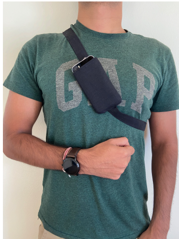
Fig. 3. In-the-wild data annotation setup using a mobile phone sitting on a strap on the chest to capture egocentric snapshots while users wore the smartwatch on the wrist.
