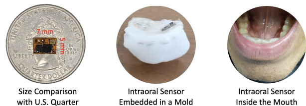
Figure 1: A sub-centimeter scale (7 mm x 5 mm) intraoral sensor was placed on a U.S. Quarter for size comparison. The device samples temperature and acceleration data at a rate of 54 Hz.
