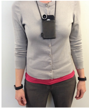
Fig. 5. Mobile phone worn on a lanyard and programmed to work as a wearable camera.
