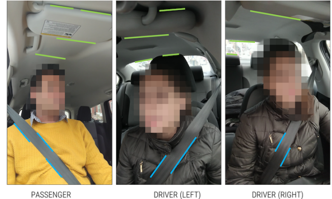
Figure 1. Lines detected in the photo captured by the phone when docked on the windshield at (a) passenger's right; (b) driver's left; and (c) driver's right side. The lines capture the perspective of the geometry of objects inside a car from different viewpoints.
