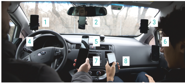
Figure 2. Different positions in which we collected the phone's camera data. The phone was docked in 3 positions on the windshield, 3 positions on the air vent, and used in the driver's hand and the passenger's hand. The users were free to switch hands as they preferred.
