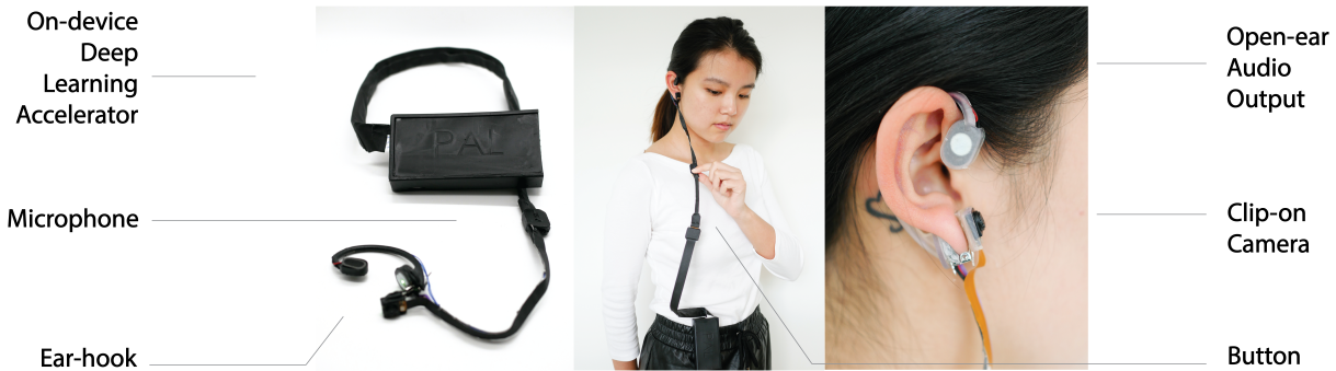
Figure 1: Wearable device with on-device deep learning, camera, open-ear audio output, microphone, and button.
