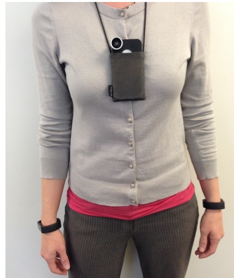
Fig. 1. The Activiome on-body sensors: a mobile phone sitting on a lanyard around the neck captures first-person photos, GPS location, inertial data from the phone’s sensors and short audio clips. Accelerometer and gyroscope data from two Movesense wearables are also collected by the Activiome mobile app.
