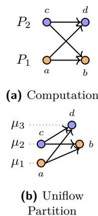
■ **Figure 6** A computation on two processes in: (a) its original non-uniflow partition, (b) equivalent uniflow partition
