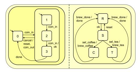
(a) Demonstrate the operation of the vending machine for a customer ordering tea. Show the sequence of events and state transitions.
