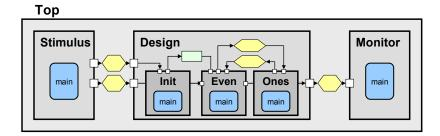
As in Problem 2.1(a), the Stimulus and Monitor modules should read the mode and the stream of input words from a file, feed them into the design over two input queues (FIFOs), receive the encoded words on an output queue (FIFO), write the result to an output file, and exit the simulation cleanly when the end of the streams has been reached.
