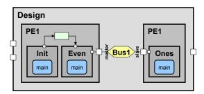
Note that in the simplest case, you can just replace all communication calls directly in the processes with equivalent calls to the corresponding bus interface methods. You are not required to implement bus drivers or bus interfaces in the PEs that translate from high-level FIFO interfaces to low-level bus read/write transactions such that no changes in the processes would be required.
