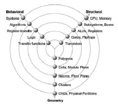
Gajski's Y chart gives the different abstractions that can be used at 3 different design views namely: Behavioral, Structural and Geometry. The outermost circle is the highest level of abstraction and the level of detail increases as we move inwards.
