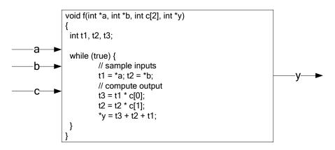
Assume a datapath resource constraint of one adder and one multiplier, where the adder requires one clock cycle while the multiplier is pipelined with a latency (delay) of two cycles and a throughput of one operation per cycle (i.e. a data introduction interval of 1).
