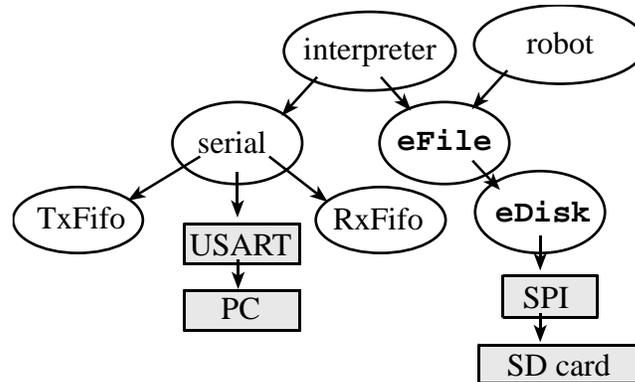
Figure 5.1. Call graph of the solid-state disk system.
