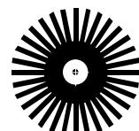
$c$  = circumference $n$  = number of slots per rotation $w$  = wheelbase $L_r = L\text{Count}^*c/n$  the arc distance traveled by the left wheel (0.01cm) $R_r = R\text{Count}^*c/n$  the arc distance traveled by the right wheel (0.01cm)
