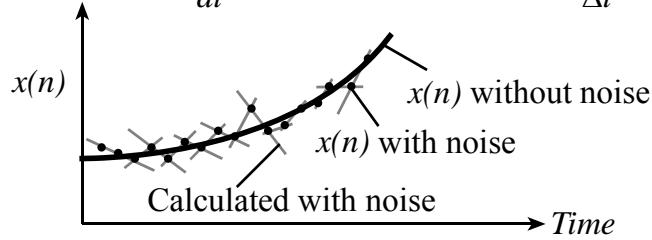
$$D(n) = K_d \left( \frac{1}{2} \frac{E(n) - E(n-3)}{3\Delta t} + \frac{1}{2} \frac{E(n-1) - E(n-2)}{\Delta t} \right) \quad \begin{array}{l} \bullet \text{Analog filter} \\ \bullet \text{Digital filter} \end{array}$$
