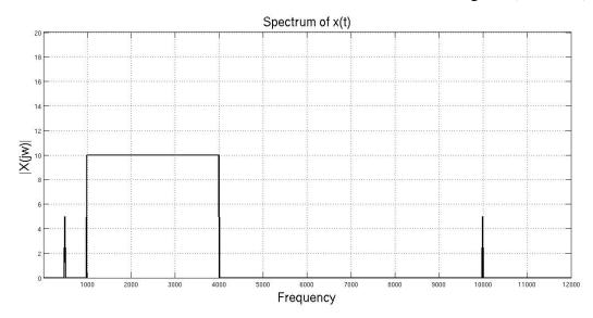
a) Choose a sampling rate (f<sub>s</sub>) for the ADC (< 12kHz) and give the cut-off frequencies of the analog low-pass filter (LPF) and of a digital filter of your choice such that x2[n] has minimal components of the interferers.
