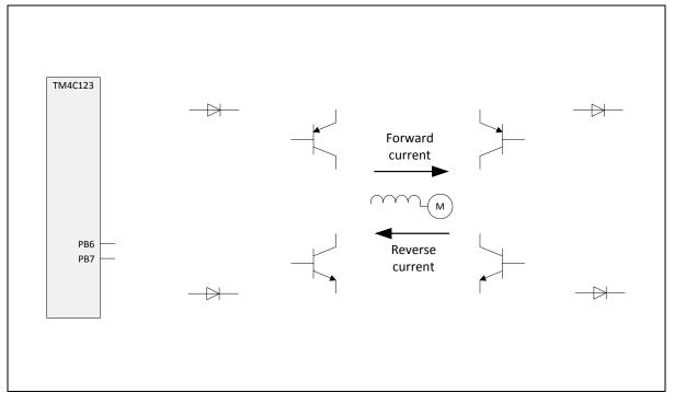
b) Show the output signals you need to create on the microcontroller's PB6 and PB7 ports to drive the motor in forward and backward direction at 1/4 of its maximum power. Also indicate (e.g. using dashed lines) how the signals would have to change to go to 3/4 power in either direction.
