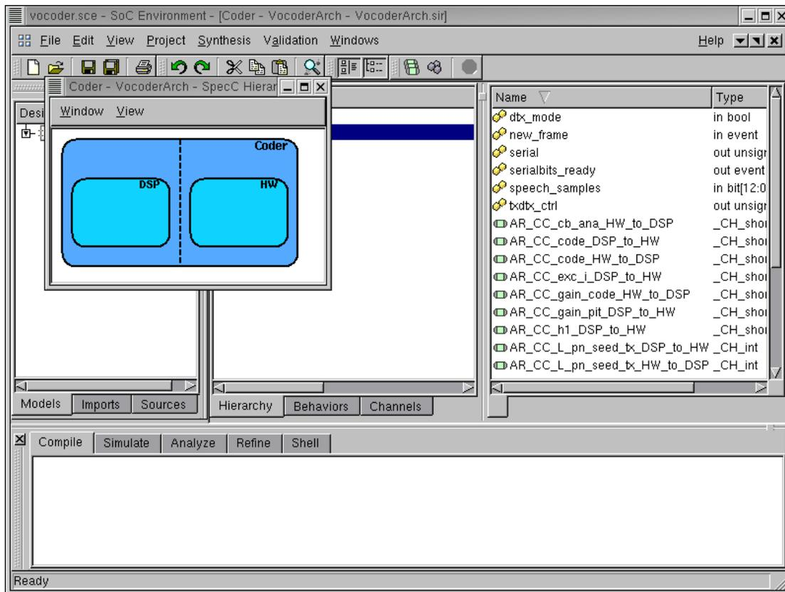
A window pops up, showing all sub-behaviors of the Coder behavior. As we can see, the top level behavior Coder in the architecture model is composed of two new behaviors, DSP and HW, which were constructed and inserted during architecture refinement. These behaviors at the top level indicate the presence of two components selected in the architecture. Note that they are also composed in parallel, which represents the actual semantics of the architecture model.
