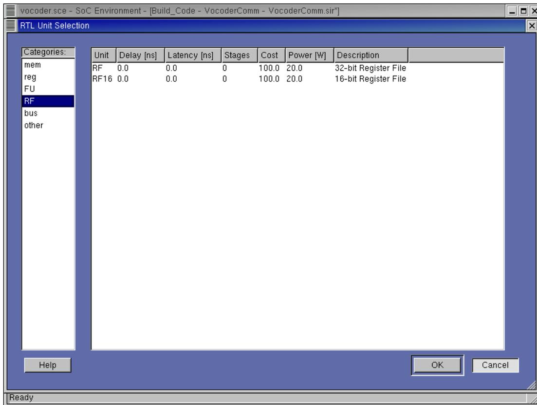
Left click on "RF" to see the various register files and their properties. Since selecting a large number of units for our example takes a lot of time, a preallocated set of RTL units may be directly imported into the design. Exit the RTL Unit Selection window by Left clicking on Cancel.
