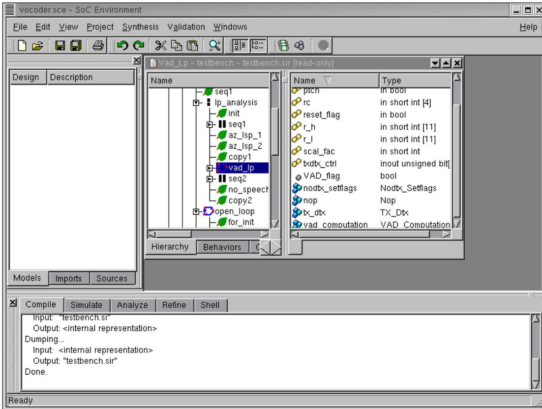
The model may be browsed using the design hierarchy window. Parallel composition is shown with || shaped icons and sequential composition with ':' shaped icons. On selecting a behavior in the design hierarchy window, we can see the behavior's characteristics in the right sub-window. For instance, the behavior "vad\_lp" has ports shown by yellow icons, variables with grey icons and sub-behaviors with blue icons.
