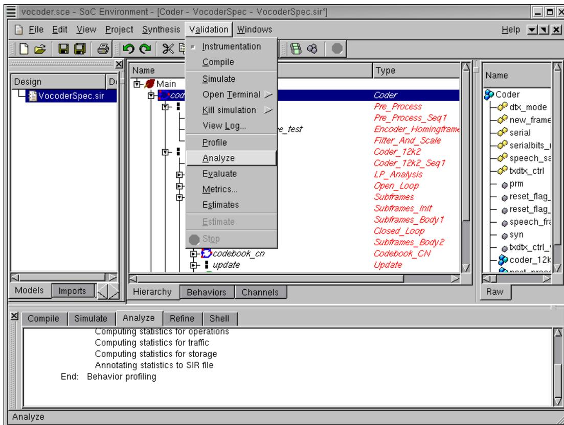
The next step is to analyze the performance of this architecture. Recall that we have a timing constraint to meet. We must therefore check if a purely software implementation would still suffice. If not, we will try some other architecture. Now we can analyze the performance of this pure software mapping by selecting **Validation** menu and select **Analyze**.
