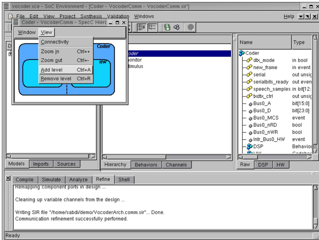
A new window pops up showing the model with DSP and HW components. We have to observe the bus controllers generated during refinement and the added details to the model. Hence, we select **View** → **Add level** from the menu bar to view the model with greater detail.
