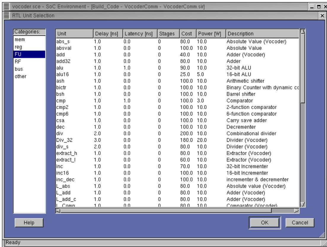
Likewise we have a set of functional units. It may be seen that the functional unit allocation must ideally comply with the profiling data. As seen during profiling, we have integer arithmetic operations in plenty. Therefore, it makes sense to allocate integer ALUs. Left click on "FU" to see the various functional units and their properties.
