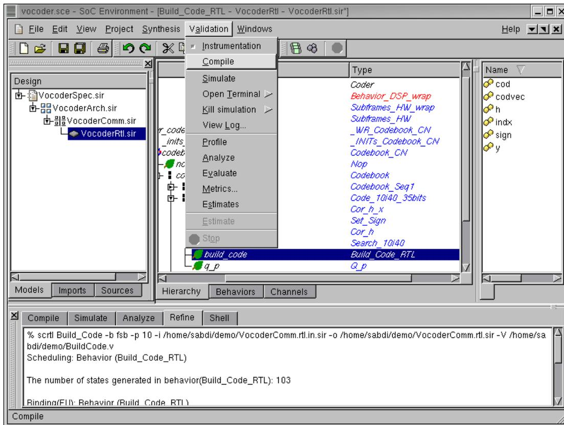
For demo purposes, we shall not perform RTL refinement on remaining behaviors assigned to HW. Proceed instead to validate the generated RTL model by selecting Validation—→Compile from the menu bar.
