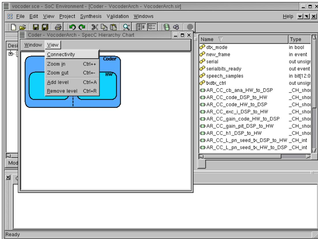
We would now like to see how the DSP and HW behaviors are communicating. This will verify if the refinement process was correctly executed. Go to **View** menu and select **Connectivity** to see the connectivity between DSP and HW components.
