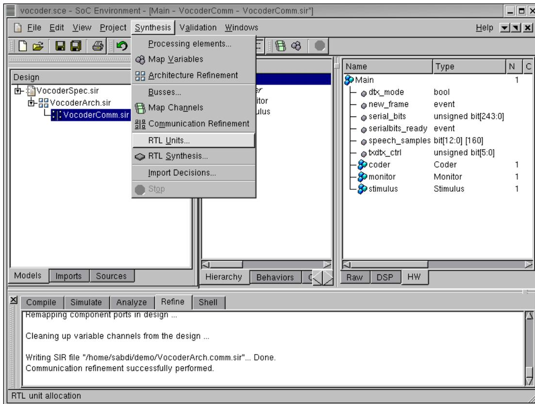
We begin RTL refinement by first verifying that the imported file has correctly allocated the RTL units. To do this, select **Synthesis**—→**RTL Units** from the menu bar.
