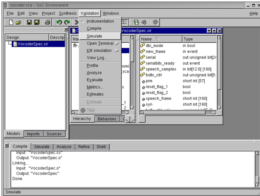
The next step is to simulate the model to verify whether it meets our requirements or not. This may be done by selecting : Validation→Simulate
