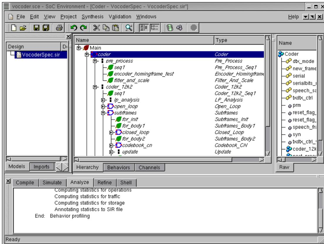
As shown in the figure, when the top level behavior *Coder* is specified, the names of all its child behaviors are italicised to distinguish them from the test bench behaviors. In general, any behavior which needs to be tested can be set as top level. So, in a generic sense, the design under test can be identified by the italicized font.
