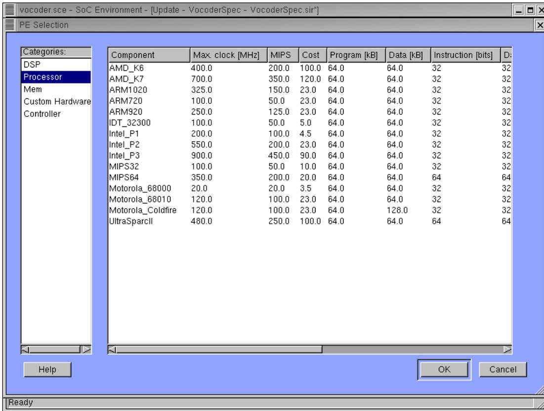
Now a PE Selection window is brought up. The left side of the window (Categories) lists five categories of components stored in the database. The right side of the window displays all components within a specific category along with their characteristics. As shown in the above figure, since the Processor category is selected on the left side, 15 commonly used processor components are displayed in detail on the right side.
