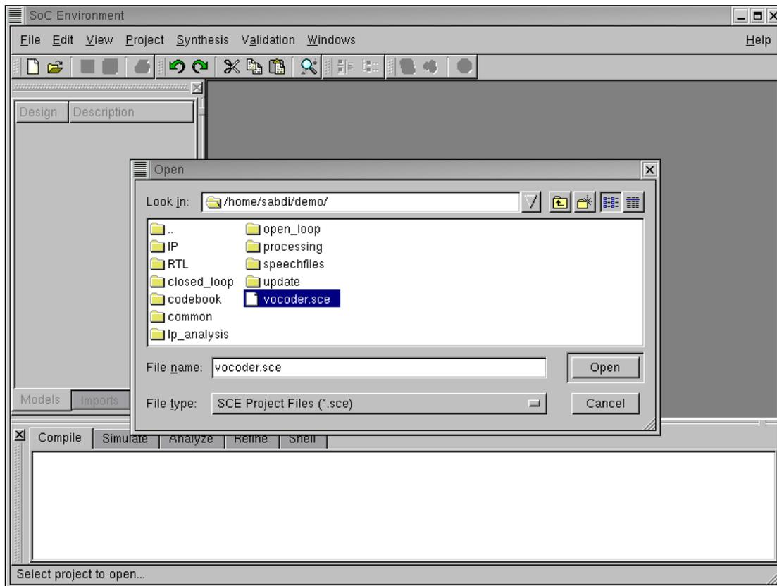
A file selection window pops up. For the purpose of the demo, a project is pre-created. We simply open it by selecting the project "vocoder.sce" and left-clicking on **Open** in the bottom right corner of the pop-up window.
