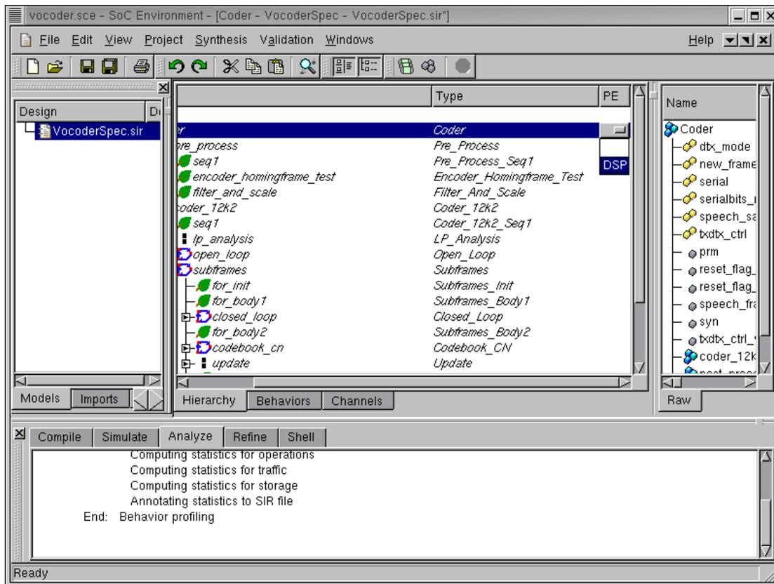
As mentioned earlier, we will map the whole design to the selected processor. This is done by assign the top level behavior `Coder` to `DSP`. Left click in the `PE` column in the row for the `Coder` behavior. A drop box containing allocated components comes up. Left click on `DSP` to map behavior `Coder` to `DSP`.
