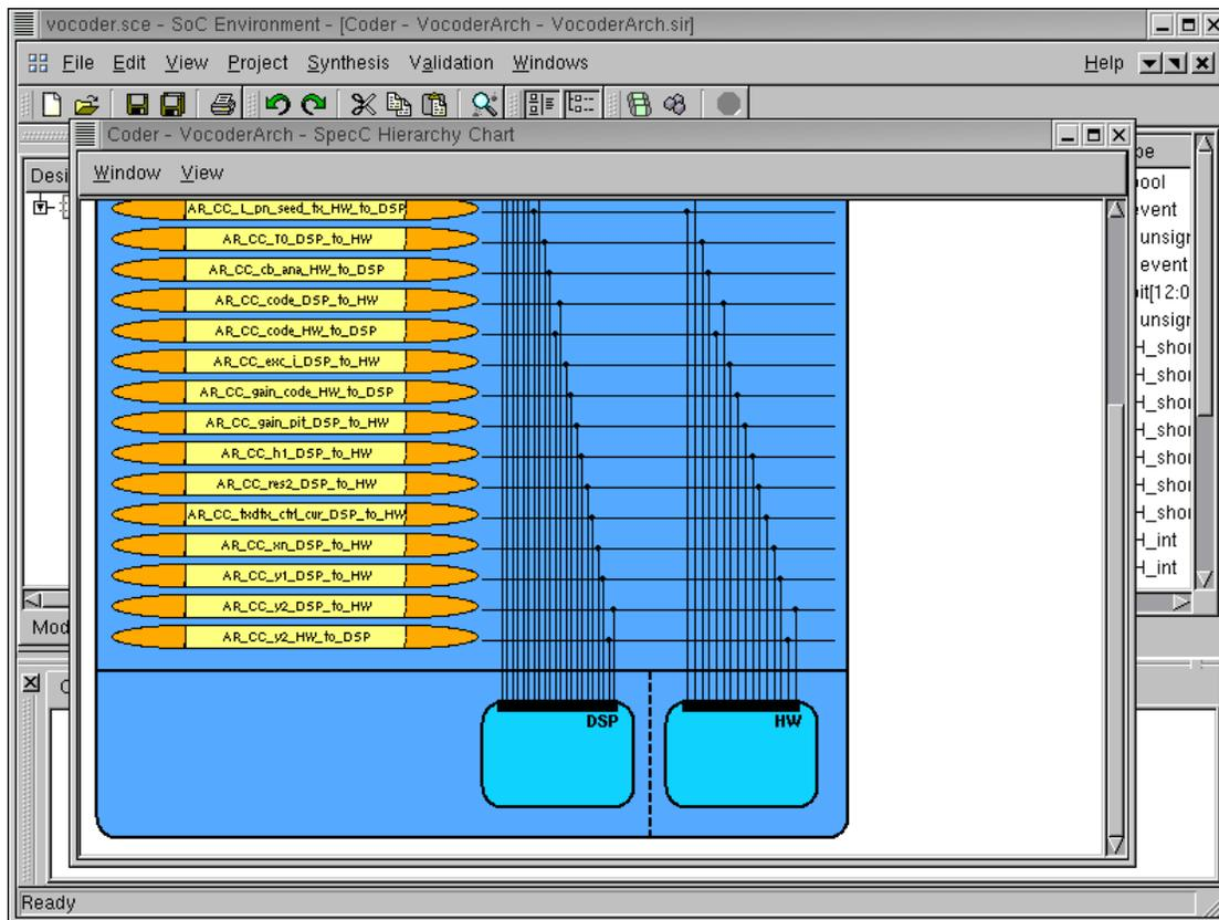
Enlarge the new window and scroll down to view the connectivity of the two components. We can see that DSP and HW components are connected through global variable channels, which were inserted during the architecture refinement. This is different from the original specification model, where only global variables were used for communication.
