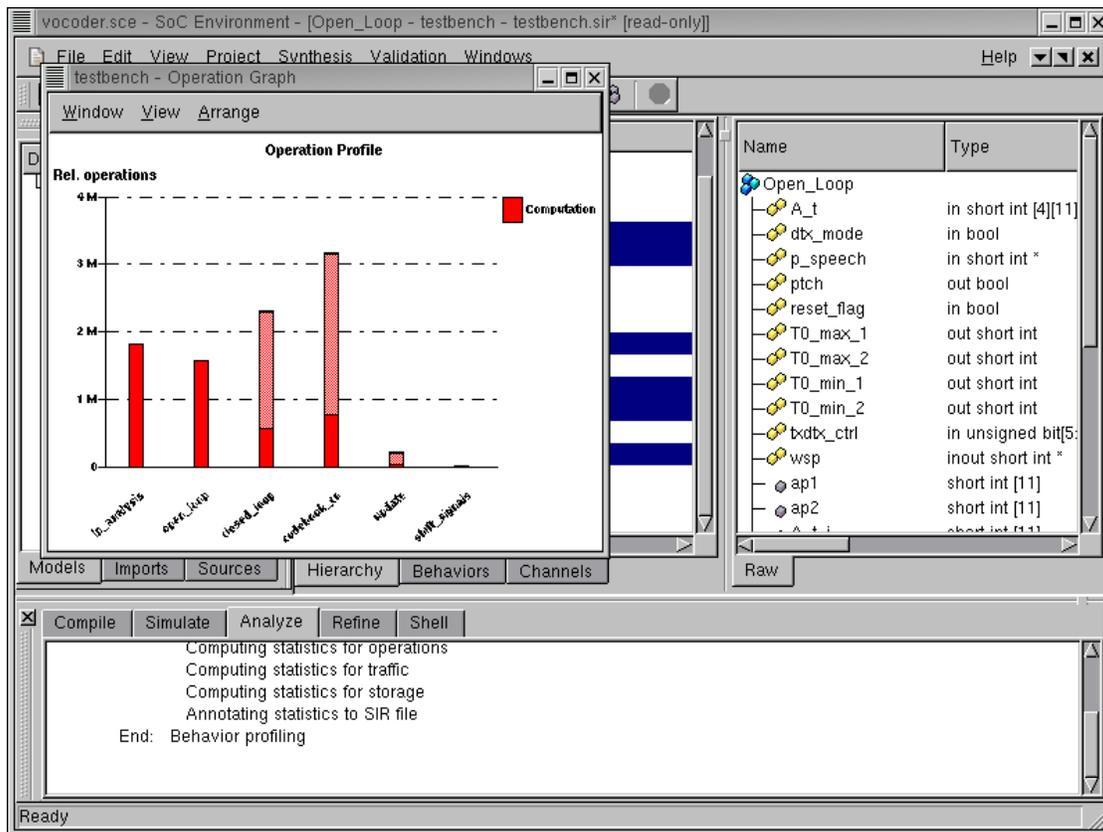
We now see a bar graph showing the relative computational intensity of the various behaviors in the selected behaviors. Essentially, the graph shows the number of operations on the Y-axis for the individual behaviors on the X-axis. Double Left click on the bar for `codebook_cn` to view the distribution of its various operations. Note that we select "codebook\_cn" because it is the behavior with the most computational complexity.
