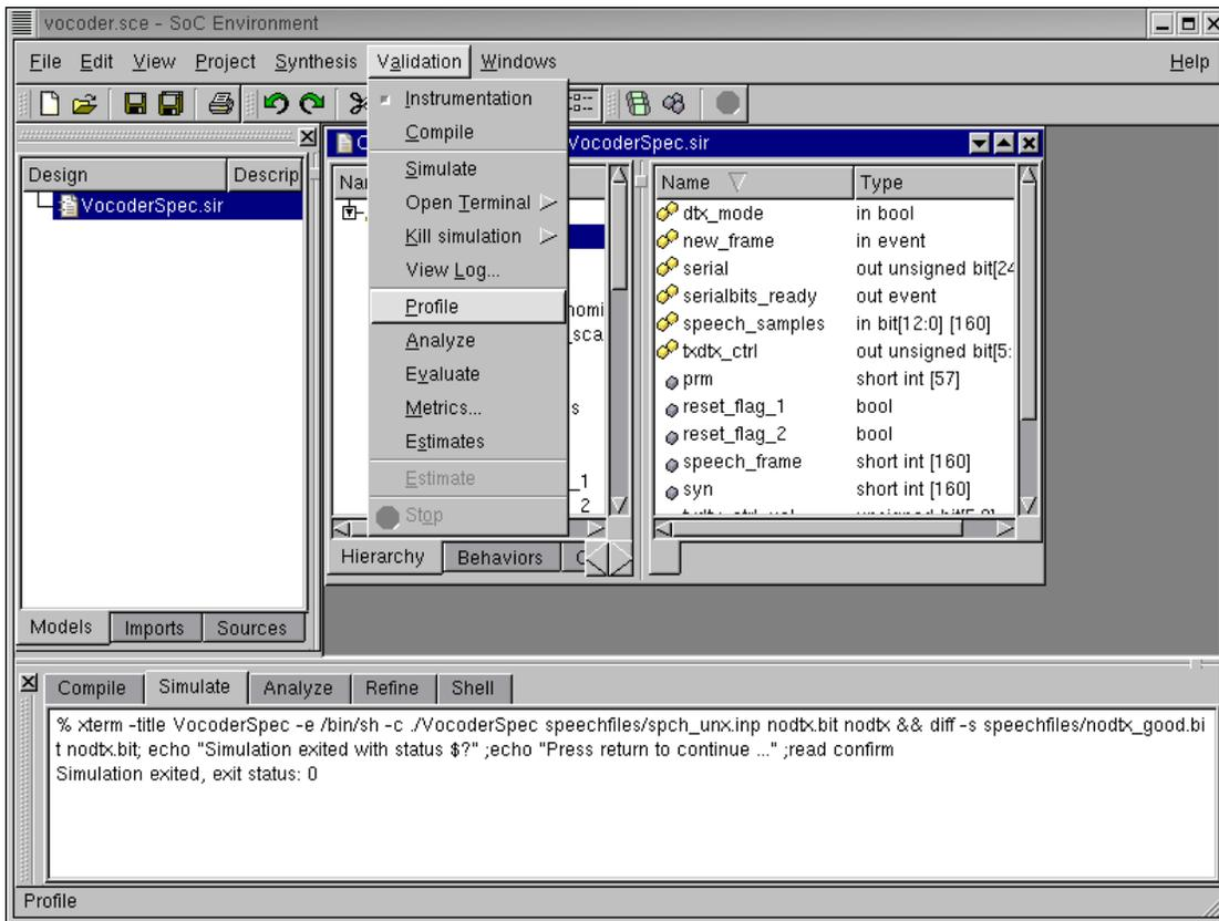
In order to select the right architecture for implementing the model, we must begin by profiling the specification model. Profiling provides us with useful data needed for comparative analysis of various modules in the design. It also counts the various metrics like number of operations, class and type of operation, data exchanged between behaviors etc. These statistics are collected during simulation. Profiling may be done by selecting : Validation→Profile
