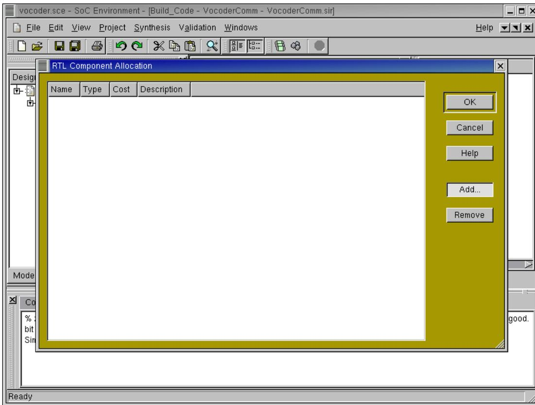
An RTL allocation window pops up just like for components and busses. Left click on Add to see the available units on the database.
