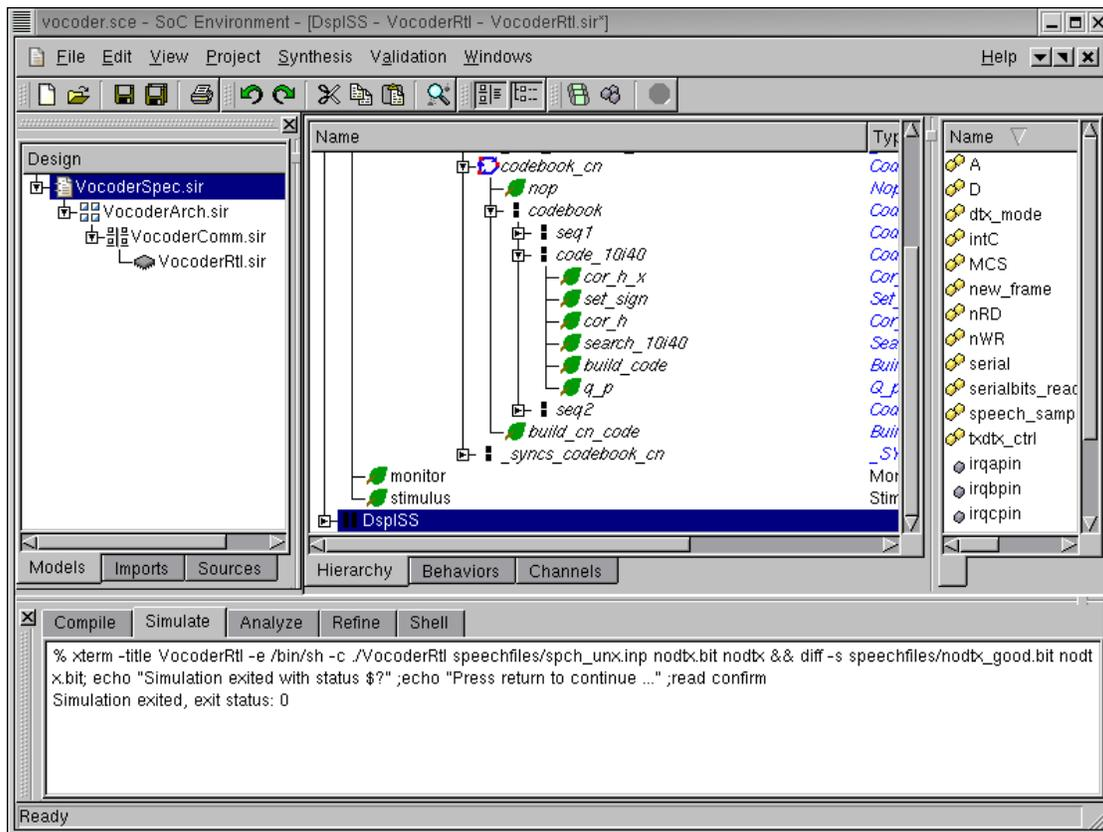
Once "DspIss.sir" is imported, we can notice DspISS as a new root behavior in the design hierarchy tree. This is because the DspISS behavior has not been instantiated yet.
