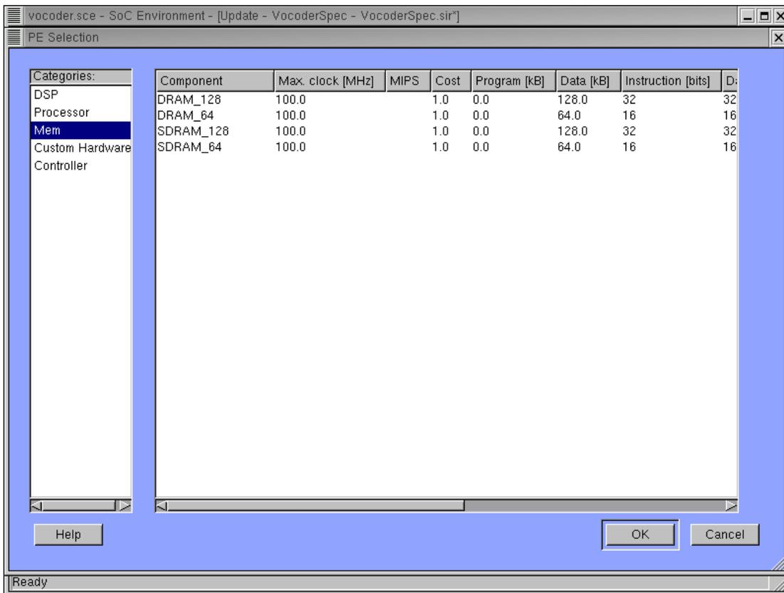
Now if we go to the **Mem** category, a number of memory components will be displayed in detail on the right side of the window. If the memory in the processor is insufficient for the application, we can add external memory components from this table.
