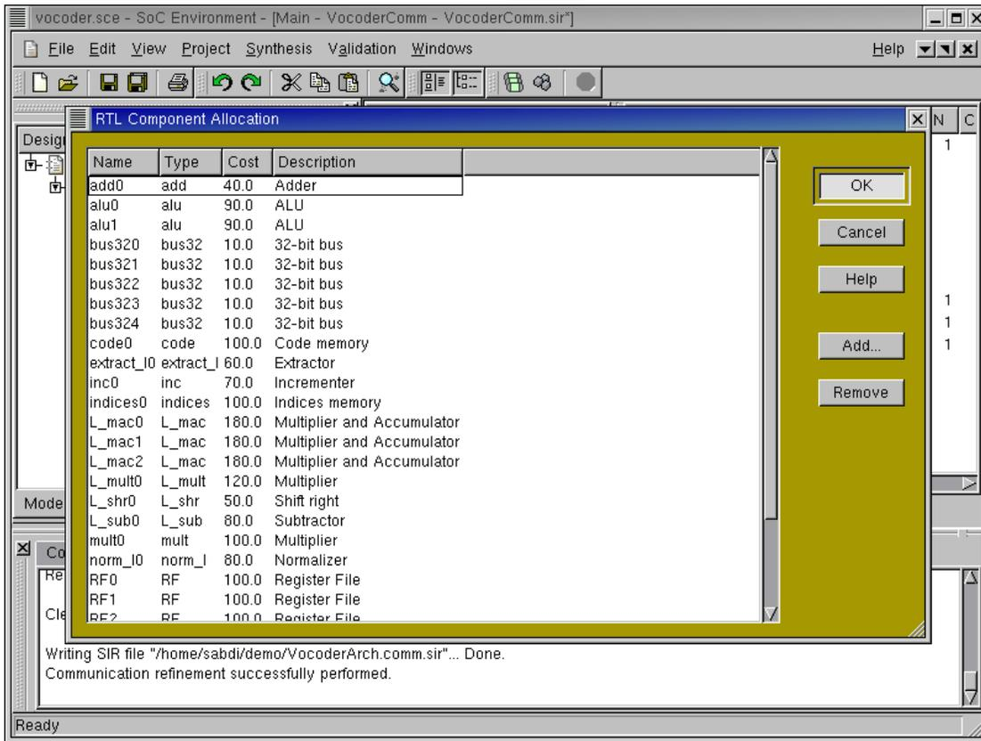
The RTL Component Allocation table pops up showing us all the allocated units. Note the presence of units for Integer arithmetic as discussed earlier. We can also see internal busses and register files in the allocation. Left click on OK to confirm the allocation.
