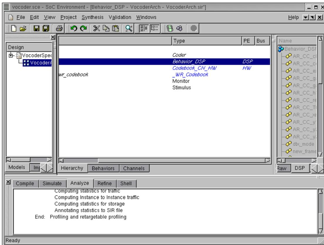
Once the bus allocation has been done, we need to group the channels of the architecture model and assign them to the system buses. Recall that in the architecture model, we had communication between components with abstract variable channels. We now have to assign those variable channels to the system bus.
