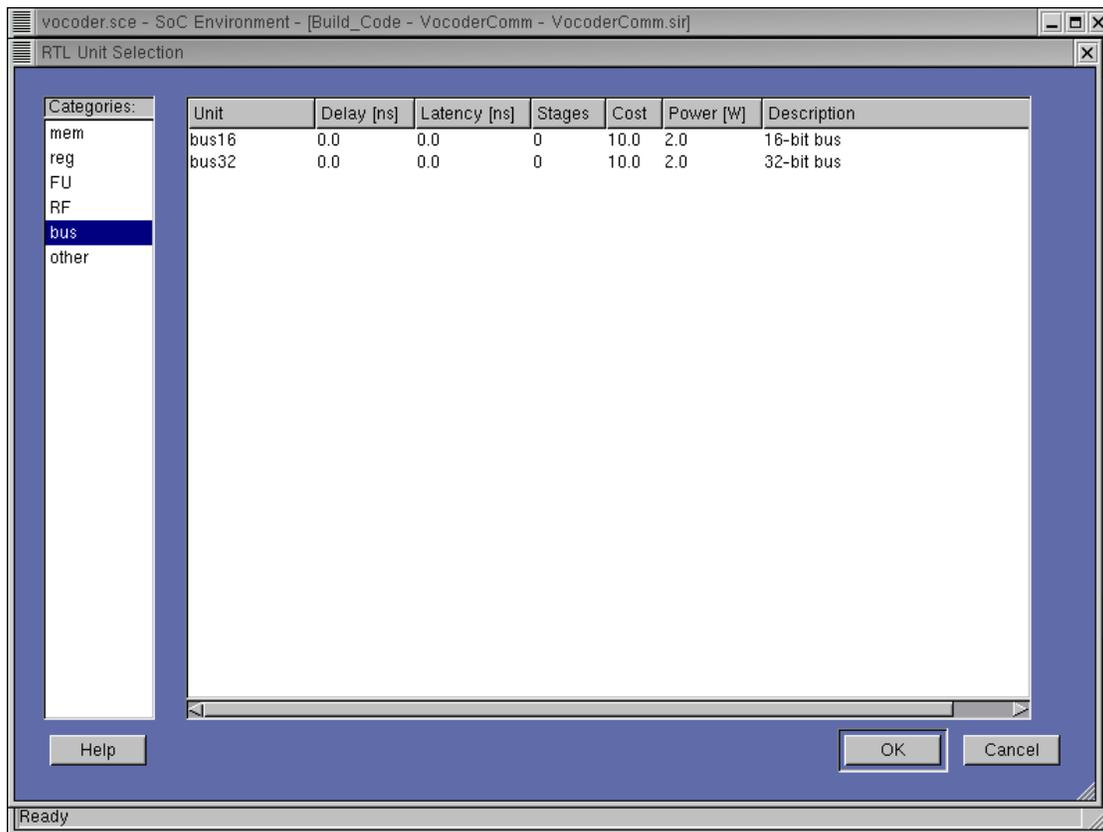
Left click on "bus" to see the available busses and their properties. These busses will be used for internally connecting the RTL units within the HW component.
