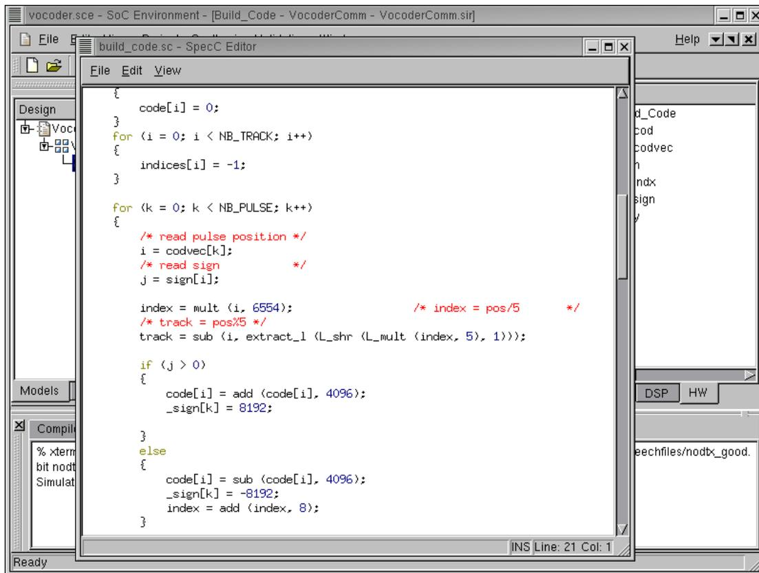
Scroll down the window to find that the behavior code has loops and conditional constructs. So, RTL refinement for this behavior will show that the tool can handle these constructs.
