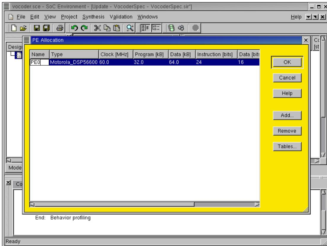
Now the PE Selection goes away and the PE Allocation table has one row that corresponds to our selected component, which has a type of Motorola\_DSP56600. This new component was named as PE0 by default. To make it more descriptive for later reference, it is desirable to rename it.
