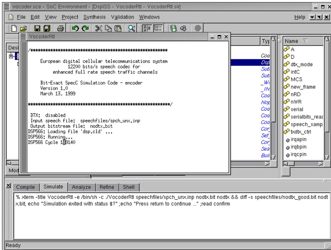
Like in the earlier cases, a simulation window pops up. The DSP Instruction set simulator can be seen to slow down the simulation speed considerably. This is because the simulation is being done one instruction at a time in contrast to the high level simulation we had earlier.
