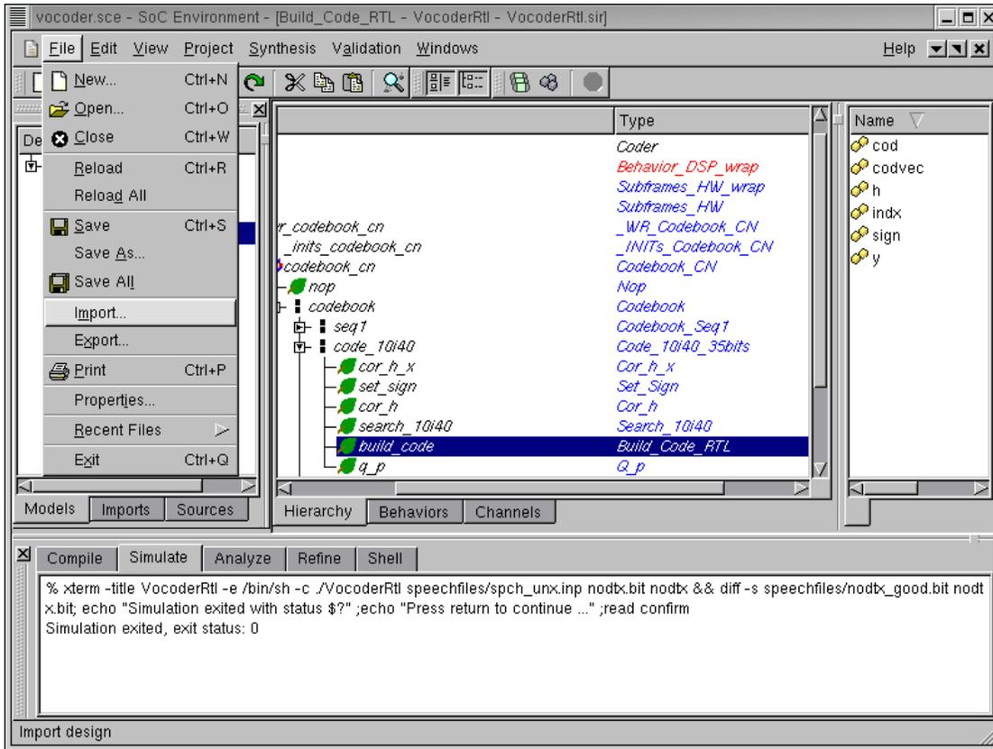
So far we have only generated the RTL model for the hardware part of our design. The behaviors that are mapped to the processor must be compiled for the DSP. We must now import the instruction set simulator (ISS) for the DSP Motorola 56600. Select **File** → **Import** from the menu bar.
