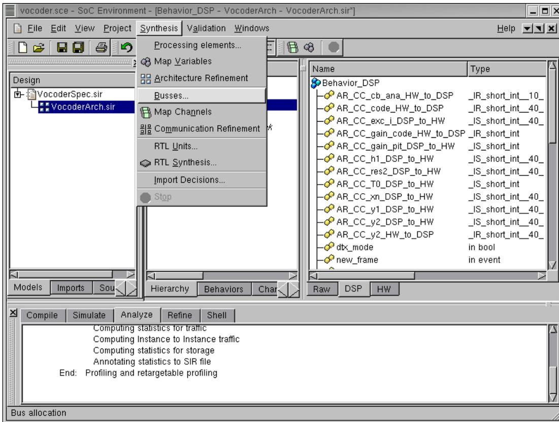
As explained earlier, we begin by selecting a suitable bus for our system. Note that in the presence of only two components, one bus would suffice. However, in general the user may select multiple buses if the need arises. Bus allocation is done by selecting **Synthesis**—→**Busses** from the menu bar.
