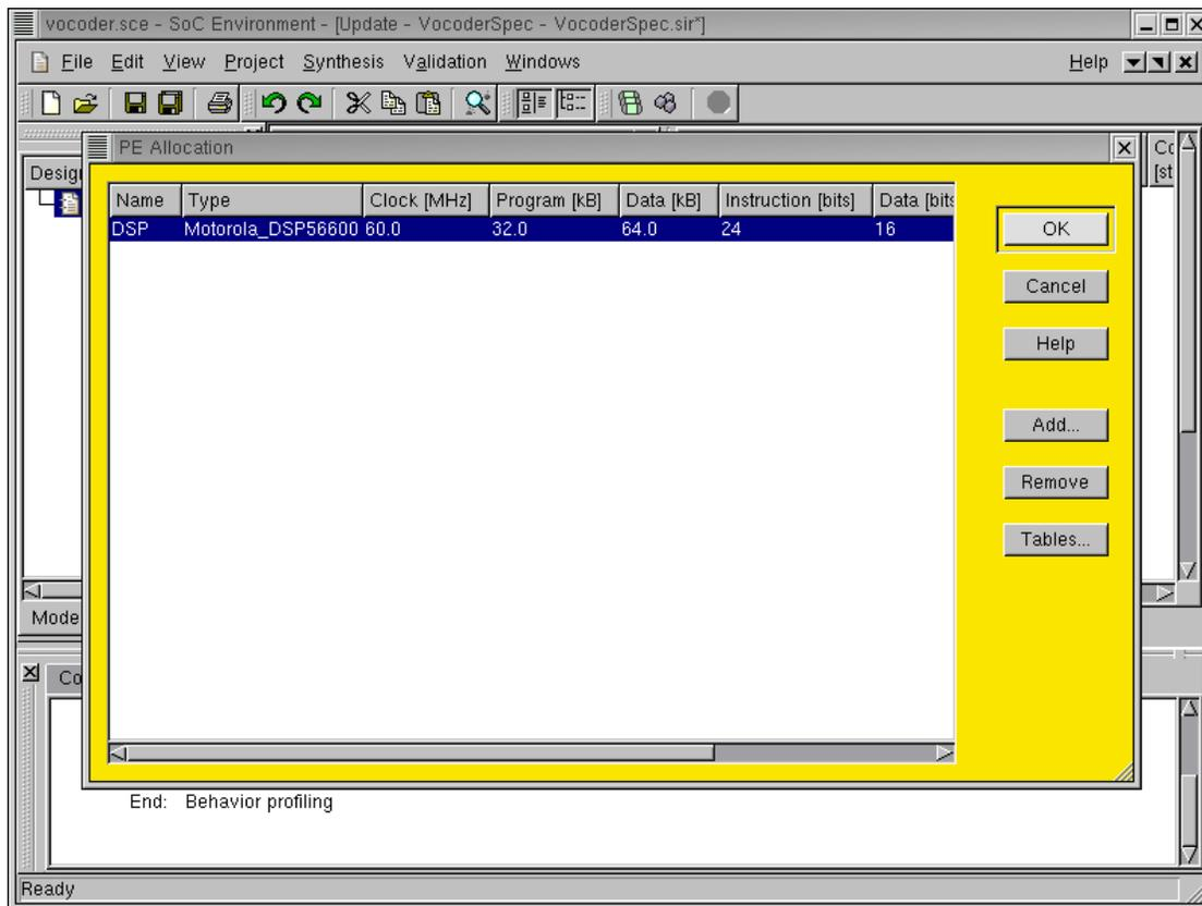
We will simply name the component as "DSP" since it is the only component used in the design at this instance. Proceed by typing "DSP" in the textfield and press return to complete the editing. Then press the **OK** to finish component allocation.
