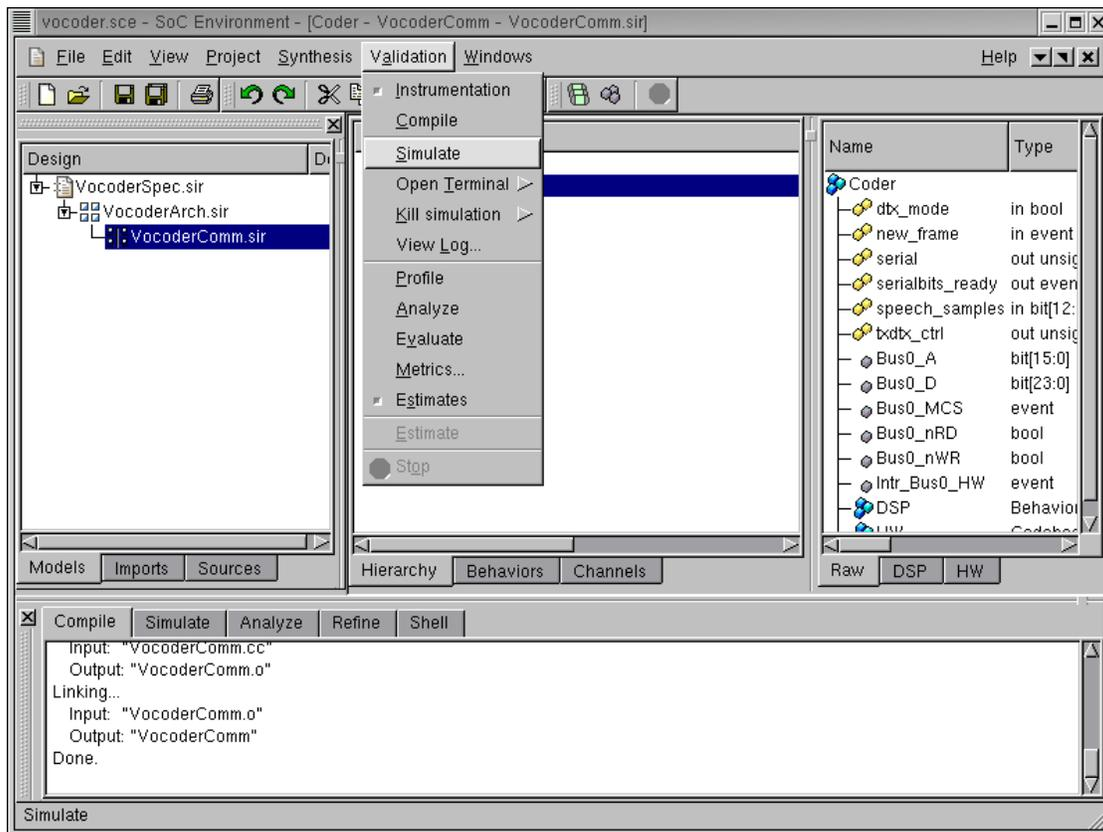
The model should compile without errors and this may be observed in the logging window. Once the model has successfully compiled, we must proceed to simulate it. This is done by selecting **Validation**—→**Simulate** from the menu bar.
