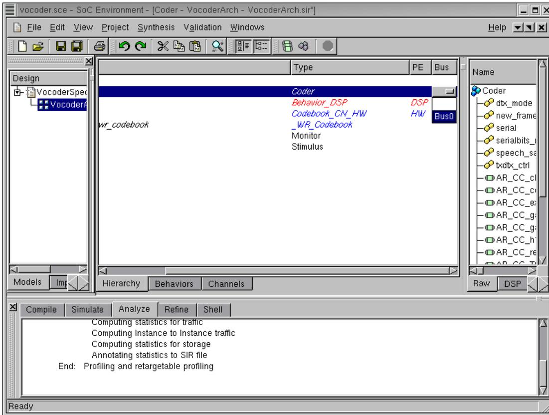
Like component mapping, bus mapping may be done by assigning variable channels to buses. However, to speed things, we may assign the top level component to our system bus. Since we have only one system bus, all the channels will be mapped to it. This is done by Left clicking in the row for the "Coders" behavior under the bus column. Select the default "Bus0" and press RETURN.
