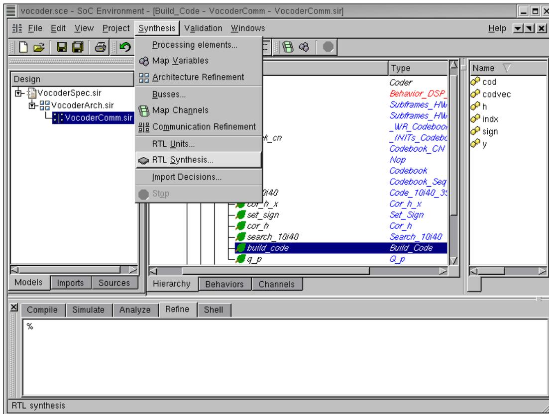
Launch the RTL refinement tool on behavior "Build Code" by selecting Synthesis→RTL Synthesis from the menu bar.
