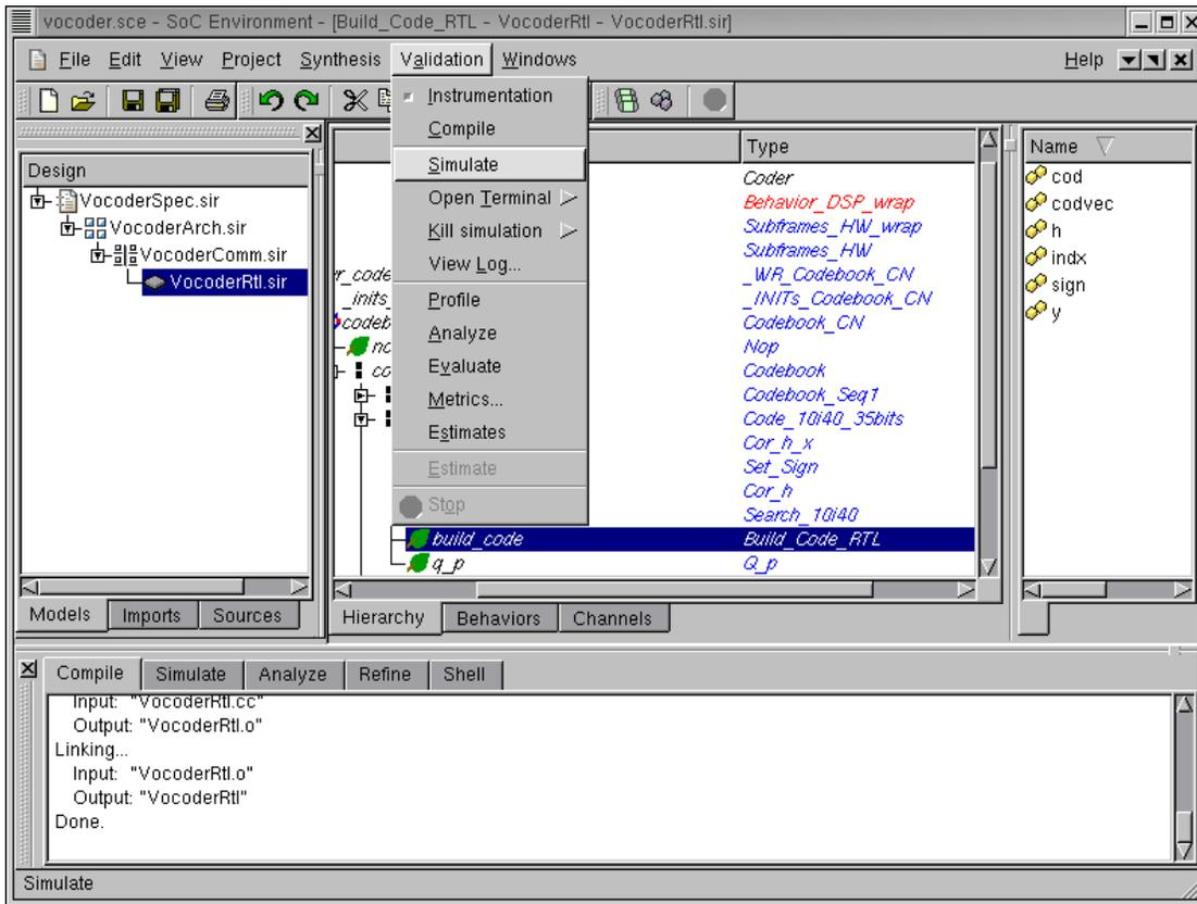
Note that the RTL model compiles correctly generating the executable VocoderRtl as seen in the logging window. We now proceed to simulate the model by selecting Validation—>Simulate from the menu bar.
