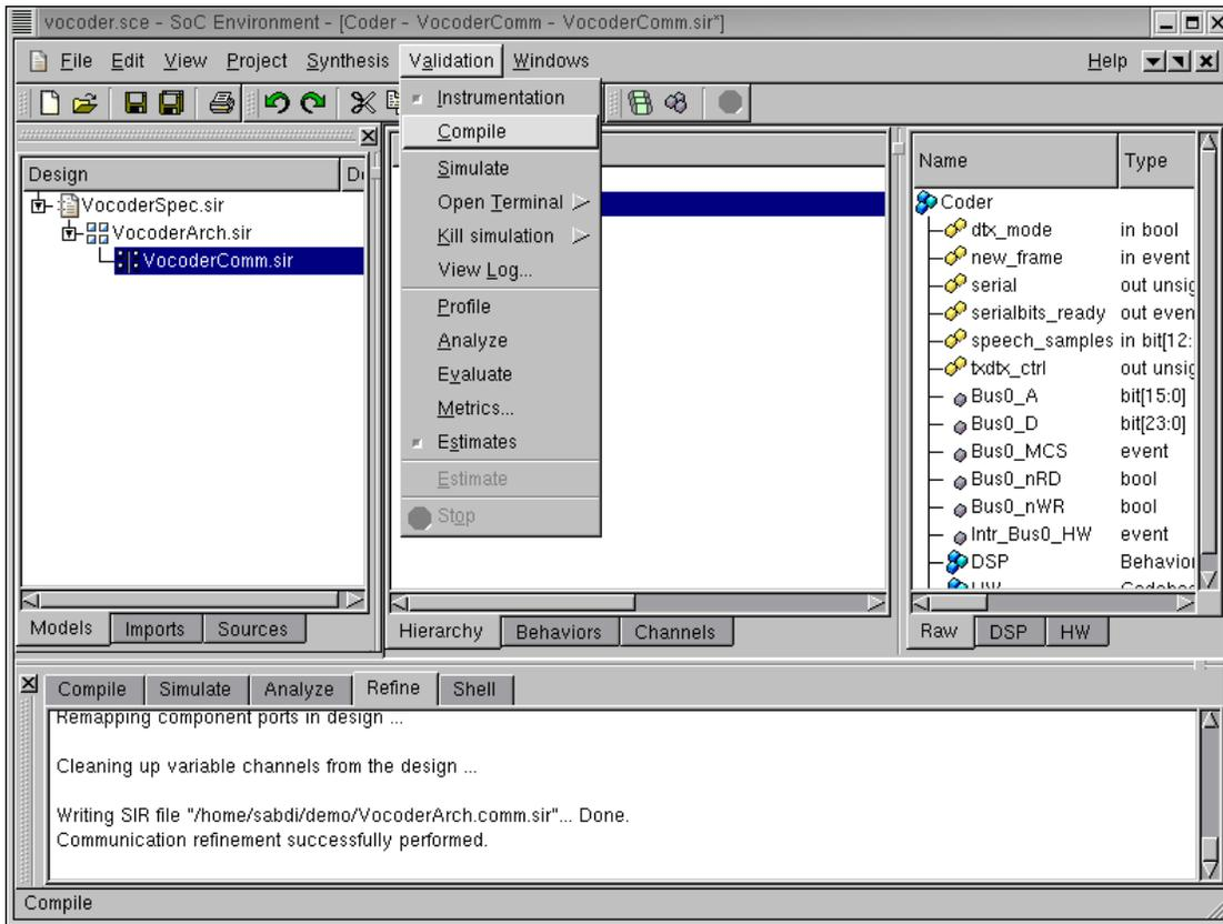
As a direct analogy to the validation of the architecture model, we have a step for validating the communication model. The newly generated model has already been verified to adhere to our notion of a typical communication model. We must now verify that the communication model generated after the refinement process is functionally correct or not. Towards this end, the model is first compiled. This is done by selecting Validation—→Compile from the menu bar.
