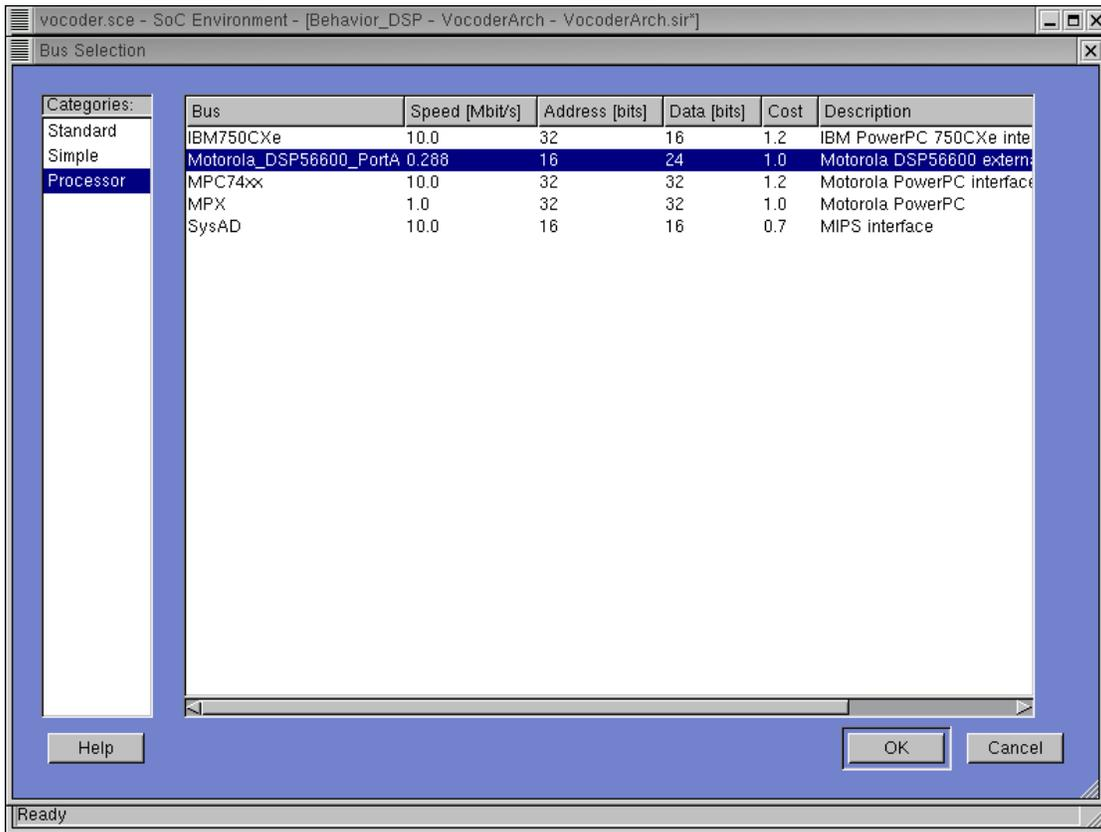
A new window pops up showing the contents of the protocol database. The column on the left shows the three categories of protocols. During component selection for architecture exploration, we had a classification of components. Likewise, the classification here shows us the available types of busses. On selecting a particular category by Left click, the busses under that category are displayed. For our demo purposes, we select the Processor bus "Motorola\_DSP56600\_PortA" and click OK.
