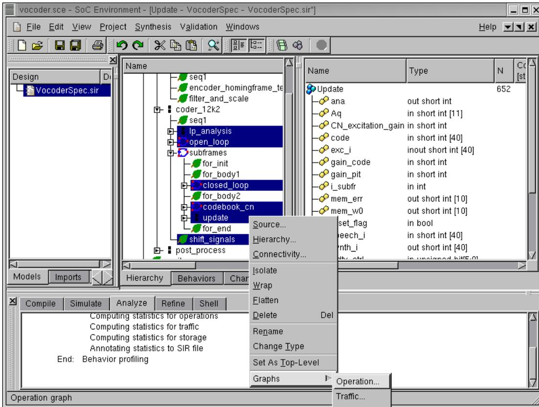
In order to select a suitable architecture for the Vocoder, we must perform not only an absolute but a comparative study of the computation requirements of the selected behaviors. SCE provides for graphical view of profiling statistics which may be used for this purpose. After the multi-selection, we Right click and select: Graphs→Operation
