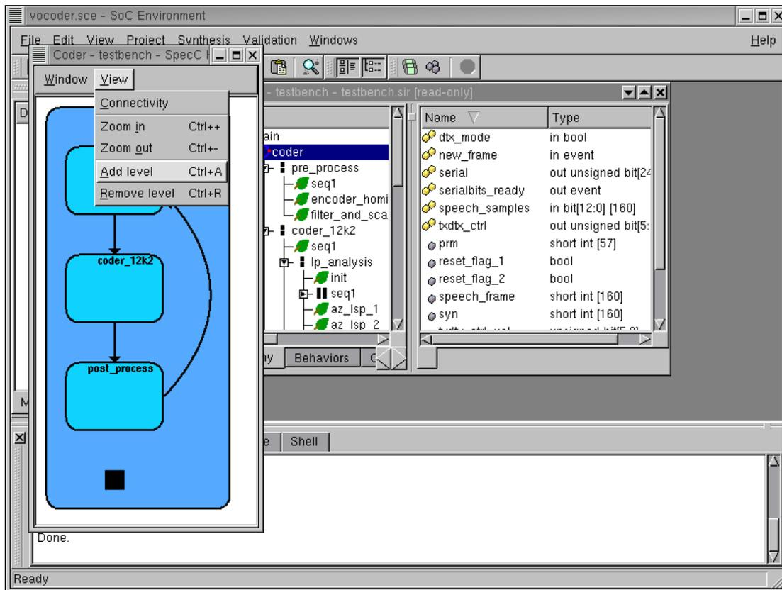
At this stage, we would like to delve into greater detail of the specification. To view the model graphically with higher detail, select **View**—→**Add level**. Perform this action TWICE to get a more detailed view. As can be seen, the **View** menu provides features like displaying connectivity of behaviors, modifying detail level and zooming in and out to get a better view.
