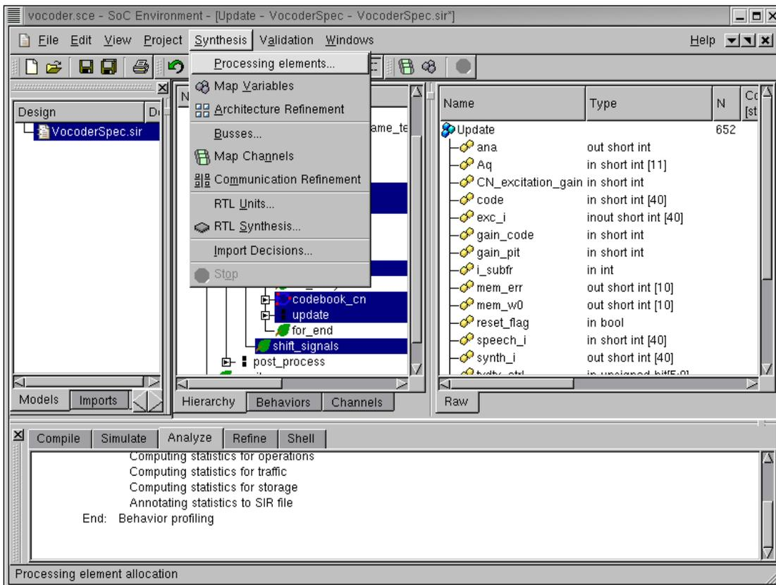
We begin by exploring the available set of components in the database. This is required to select a suitable processor. To view all available components and select the desired processor, go to the **Synthesis** menu on the menu bar and select **Processing elements**.
