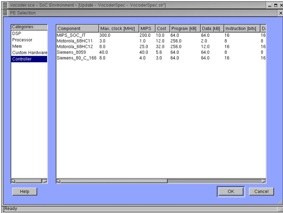
Now if we go to the **Controller** category, a number of widely used microcontroller components will be displayed in detail on the right side of the window.
