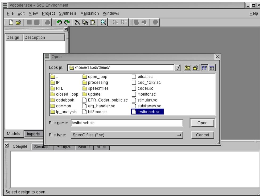
A new window pops up showing the available source files of the GSM Vocoder design specification. Select the file containing the top hierarchy of the model. In this case, the file is "testbench.sc." The testbench instantiates the Design under Test (DUT) and the corresponding modules for triggering the testvectors and for observing the outputs. To open this file Left click on Open.
