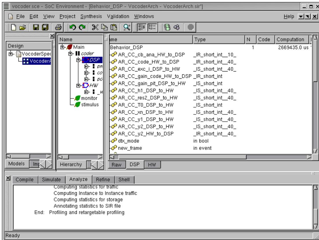
As we can see in the logging window, a profiling retargeted at the DSP is being performed. When it finishes, the profiled data is presented in the design window. Clicking DSP in the hierarchy tree, we find out that the execution of software part (behavior Behavior\_DSP ) takes 2.67 seconds.
