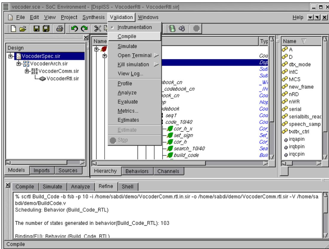
We now have the clock cycle accurate model ready for validation. We begin as usual with compiling the model by selecting **Validation**—→**Compile** from the menu bar.
