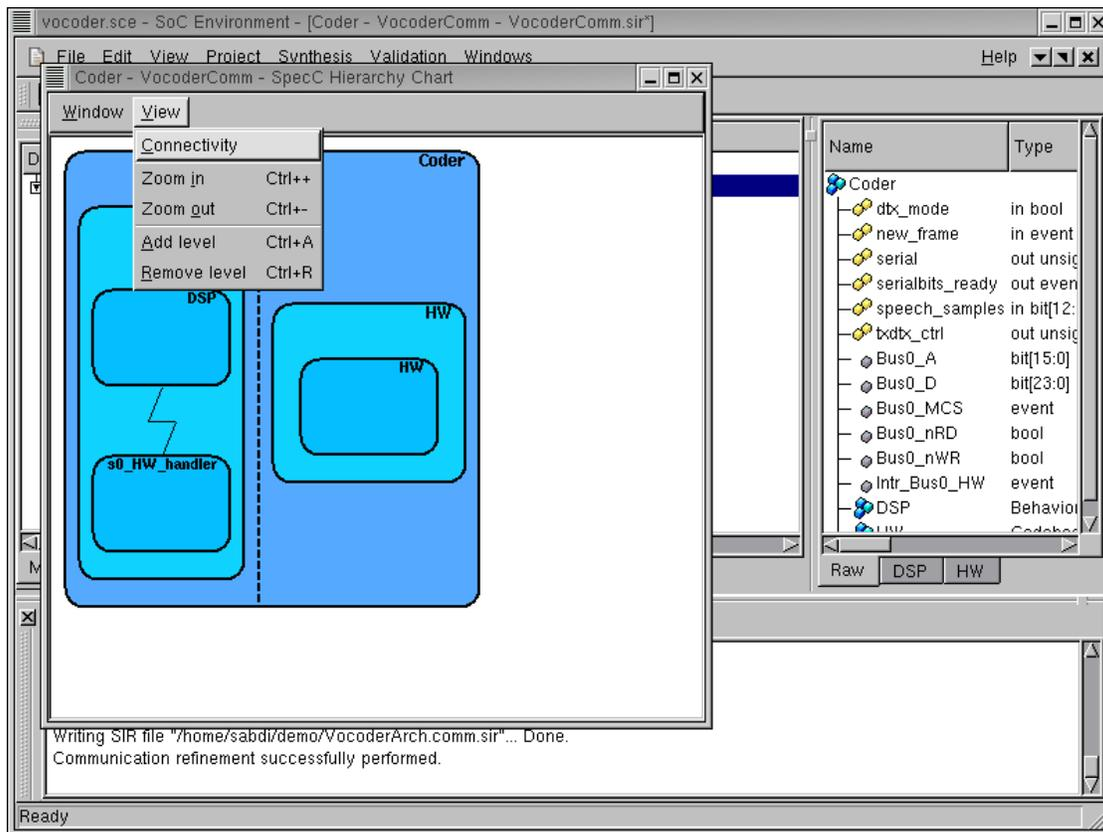
In the next level of detail, we can now see the interrupt handler "s0\_HW\_handler" behavior added in the master to serve interrupts from the HW slave. To view the actual wire connections of the system bus, enlarge window and select **View**→**Connectivity** from the menu bar.
