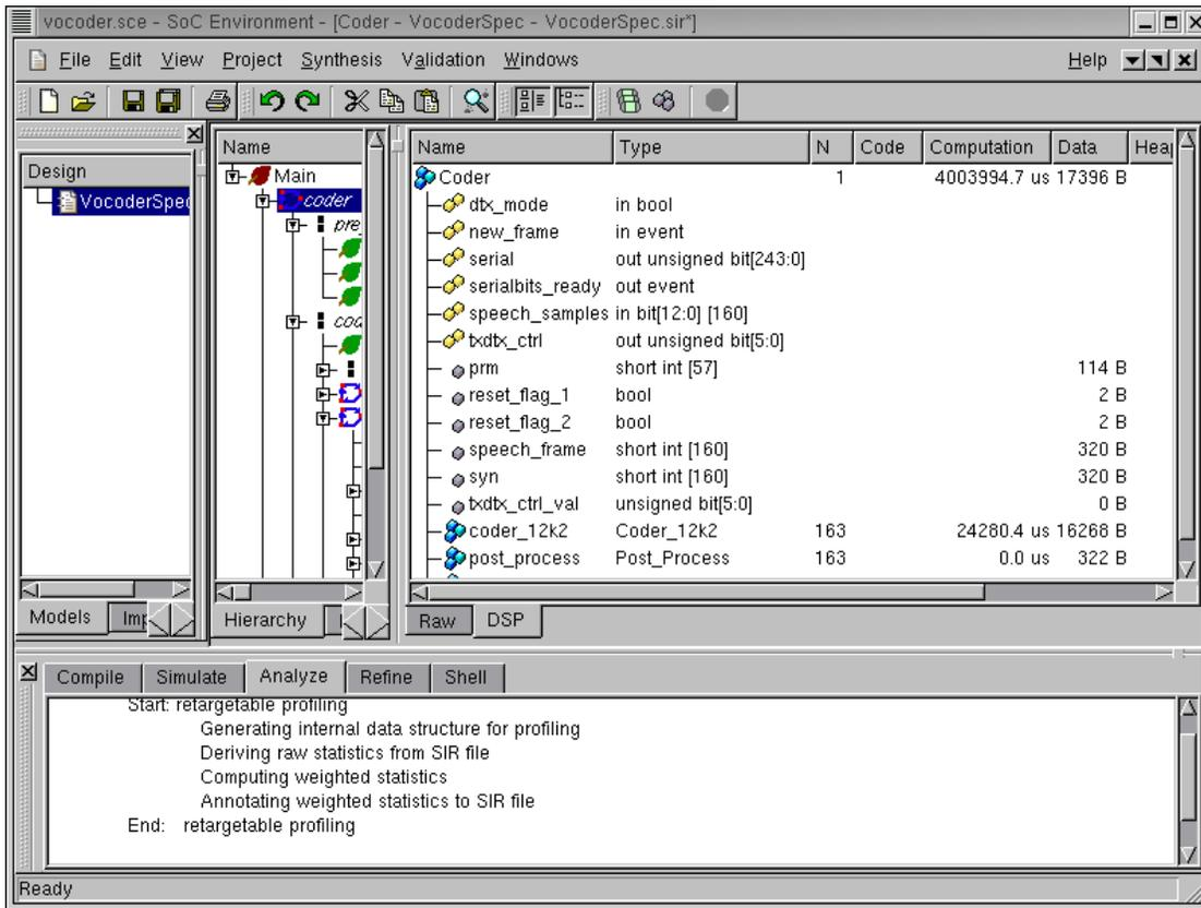
As seen in the design window, the computation time is in terms of `us`. As we can see in the row of behavior `Coder`, the estimated execution time ( $\sim 4.00$  seconds) exceeds the timing constraint of 3.26 seconds. Therefore, the pure software solution with a single `Motorola_DSP56600` does not work. We, therefore, need to experiment with other architectures.
