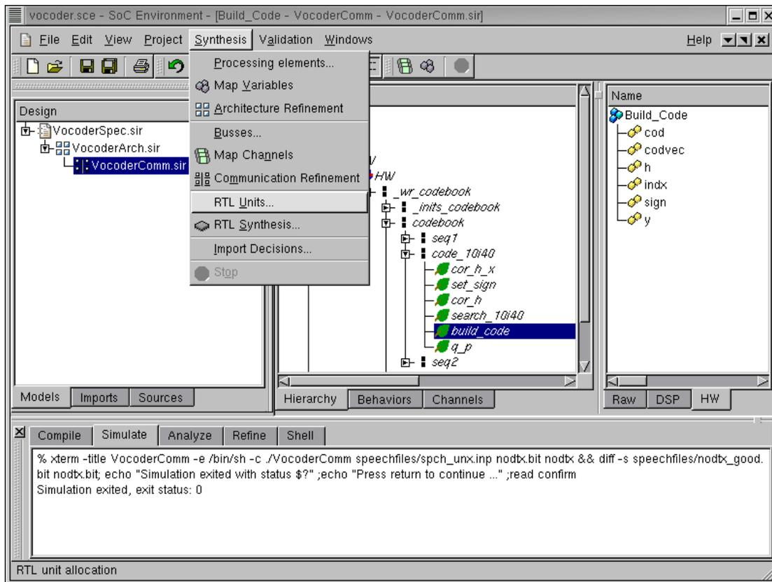
In order to perform refinement, we need to have RTL units that will be used to generate the structural RTL model. The next step is thus to select RTL units for allocation. To perform the allocation select **Synthesis**→**RTL Units** from the menu bar.
