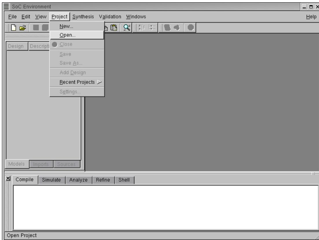
The first step in working with SCE is opening a project. A project is associated with every design process since each design might impose a different set of databases or dependencies. The project is hence used by the designer to customize the environment for a particular design process. We begin by selecting **Project**—→**Open** from the menu bar.
