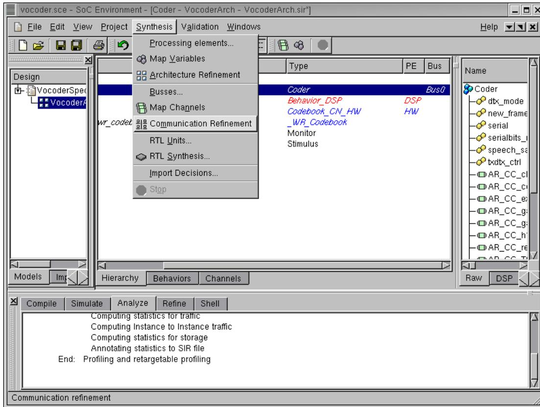
Now that we have completed bus allocation and mapping, we may proceed with communication refinement. Like architecture refinement, this process automatically generates a new model that reflects our desired bus architecture. To invoke the communication refinement tool, select **Synthesis** → **Communication Refinement** from the menu bar.
