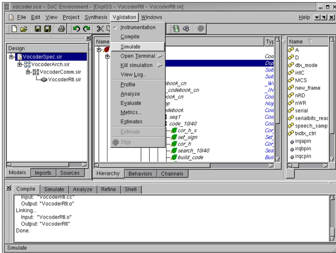
The model compiles correctly as shown in the logging window. We now proceed to simulate the model by selecting Validation→Simulate from the menu bar.
