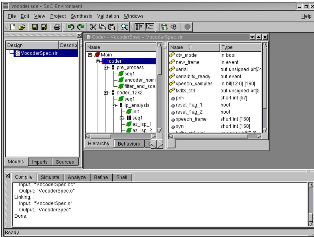
Note that in the logging window we see the compilation messages and an output executable "VocoderSpec" is created.
