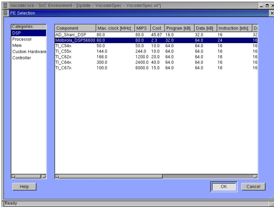
Through earlier profiling and analyzing, we found out that integer multiplication is the most significant operations in the original specification. Therefore, a fixed-point DSP would be desirable for this design.
