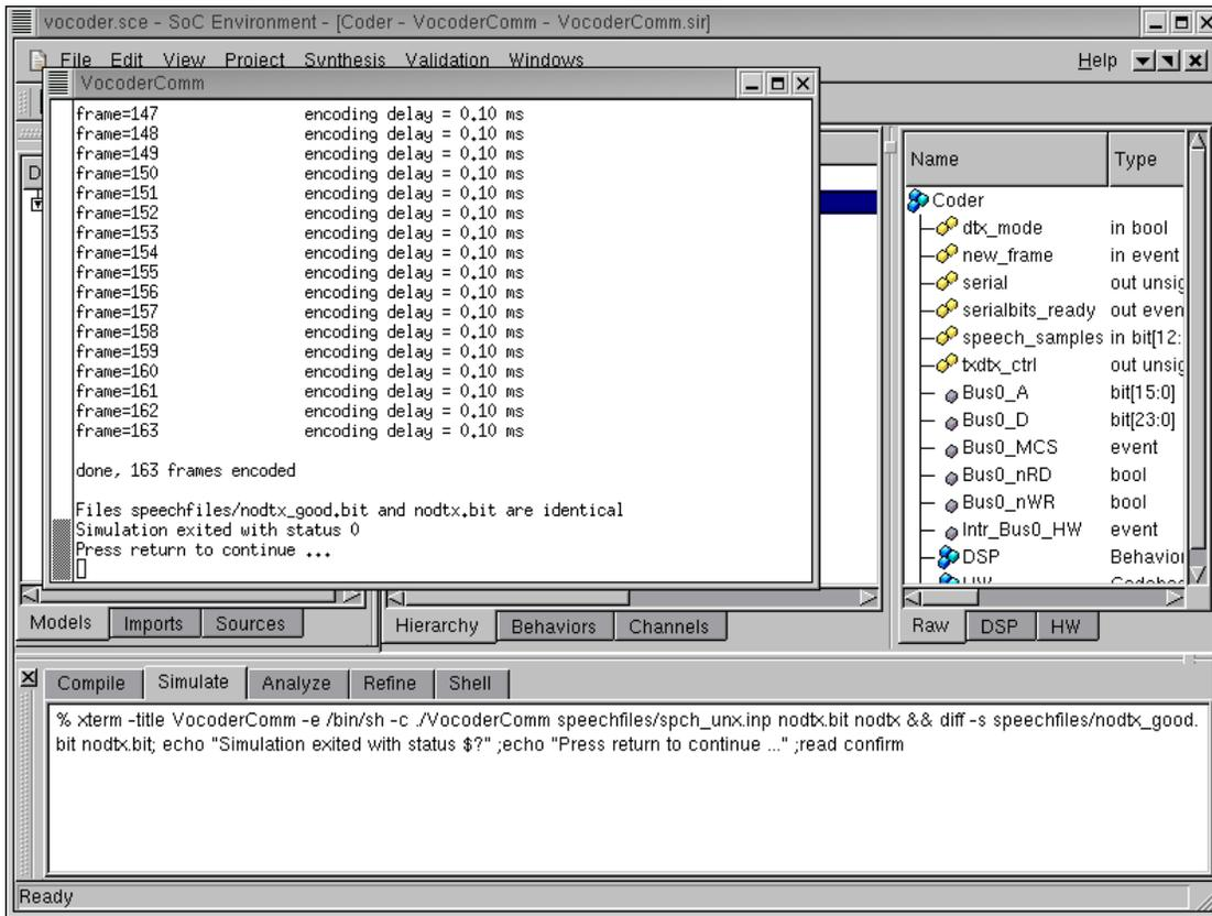
An xterm now pops up showing the simulation in progress. Note that simulation is considerably slower for the communication model than for the architecture and communication model. This is because of the greater detail and structure added during the refinement process. Also, it may be noted that there is non-zero encoding delay. This is because the new model is timed and takes into account the delay caused during computation and communication.
