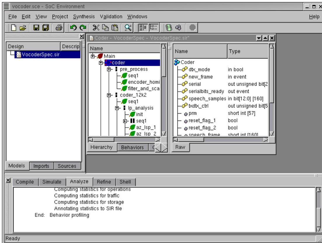
The logging window now shows the results of the profiling command. Note that there is a series of steps for computing statistics for individual metrics like operations, traffic, storage etc. Once these statistics are computed, they are annotated to the model and displayed in the design window.
