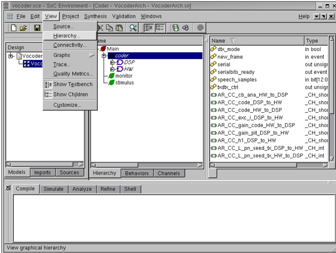
Since the top level behavior is **Coder**, the test bench behaviors are not changed during architecture refinement. Therefore let's select the **Coder** by clicking in the corresponding row in the design window. We would like to see how the design looks when it is mapped to the selected architecture. To view the hierarchy of the new **Coder** behavior, go to **view** menu and select **Hierarchy**.
