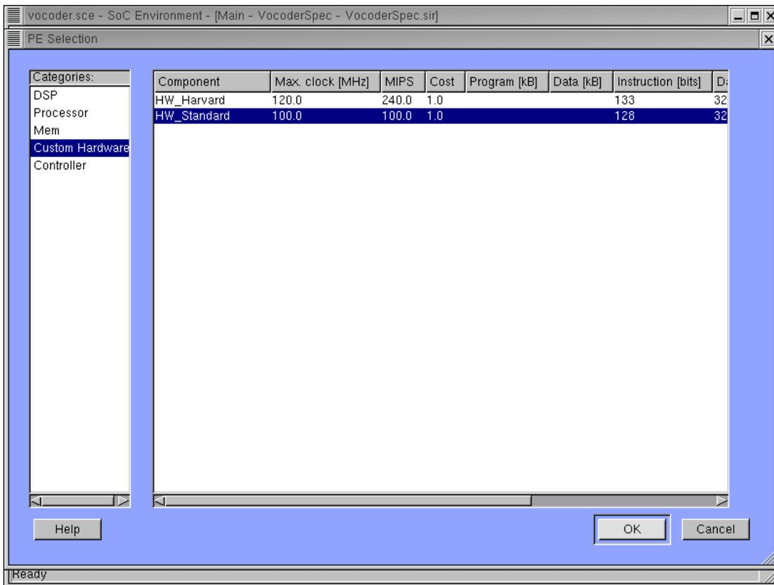
In the **Custom Hardware** category, two general types of hardware components are displayed. Here we will use the standard hardware design with a datapath and a control unit. Select the **HW\_Standard** and press **OK** to confirm the selection.
