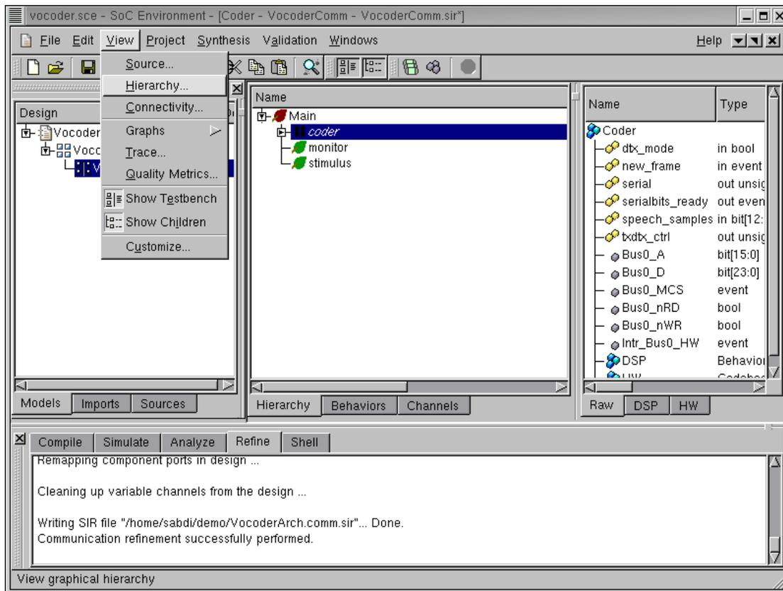
Like we did after architecture refinement, we browse through the communication model generated by the refinement tool. We have to first check whether it is semantically and structurally representing a model as described in our SoC methodology. To observe the model transformations produced by communication refinement, we need a graphical view of the model. This is done by Left clicking to choose the "Coder" behavior in the design hierarchy window and selecting View → Hierarchy from the menu bar.
