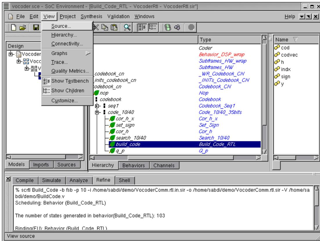
Select the behavior "Build\_Code\_RTL" by Left clicking on it. We now take a look at the synthesized source code to see if the RTL refinement tool has correctly generated the RTL model. Do this by selecting **View**→**Source** from the menu bar.
