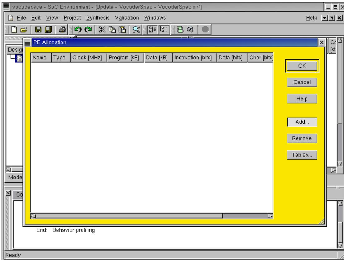
Now a **PE Allocation** window pops up. This window includes a table to display important characteristics of components selected for the design. In addition, it also provides a number of buttons (on the right side) for user actions, such as adding a component, removing a component, and so on. Since we have not allocated any component at this point, the table has no entry.
