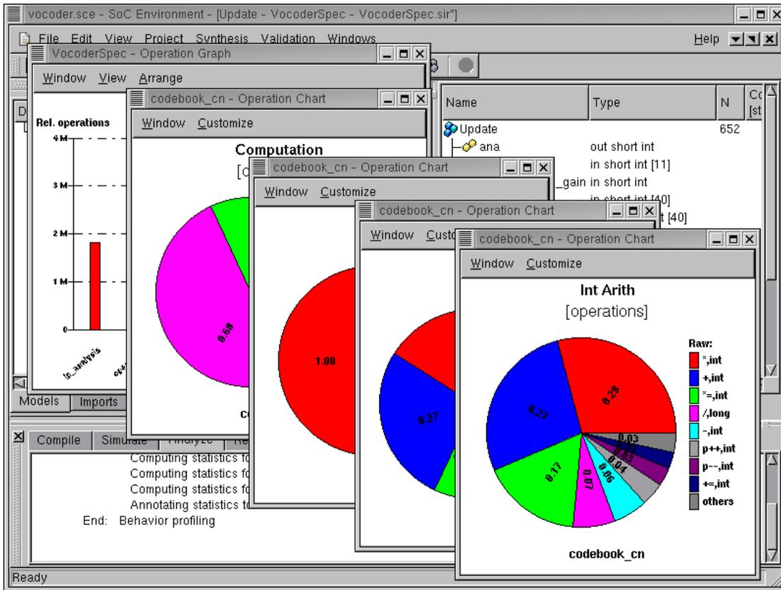
We can now observe the distribution of arithmetic operations like "multiplication", "addition", "increment", "decrement", etc. on a new pie chart. Note that 3/4 ths of the operations are additions or multiplications, thus it would be a good idea to have these two operations directly supported by a specific hardware unit.
