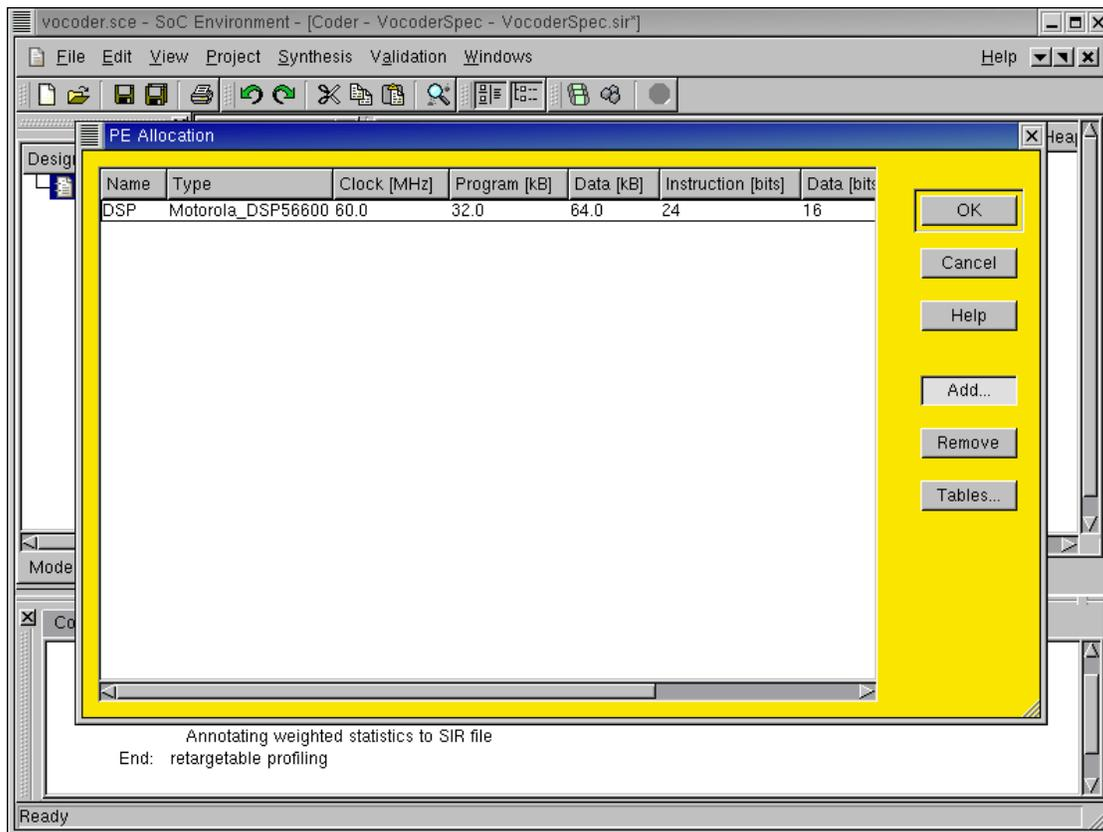
This time, the PE Allocation table pops up. As we can see, the previously allocated DSP is displayed. To insert the hardware component, press Add button to go to our database.
