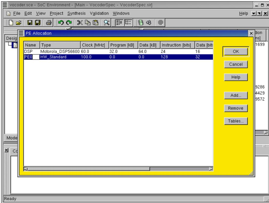
Now the HW\_Standard component is added to the PE Allocation table. In the same way we did for the DSP component, we simply rename it to "HW" to distinguish it. Notice that for the hardware component, some metrics are flexible. For instance, the clock period may be changed. However, we stay with the current speed of 100 Mhz for demo purpose.
