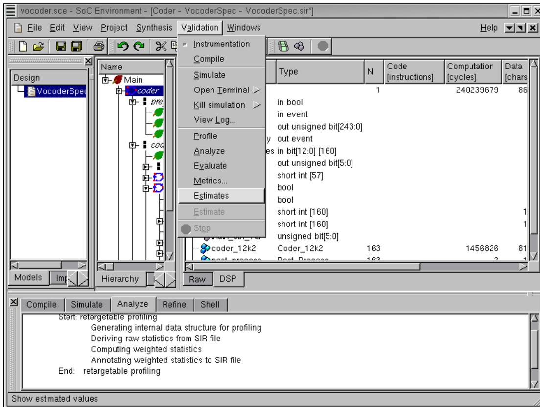
The number of computation cycles is a relevant metric for observation. However, it must be converted to an absolute measure of time so that we may directly verify if this architecture meets the demands. To find out the real execution time in terms of seconds, we turn on the option for estimation as follows. Go to **Validation** menu and select **Estimates**.
