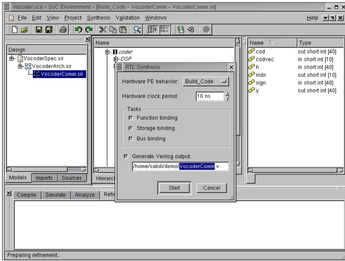
In the newly popped up window, change the name of the generated verilog file to "Build-Code.v" so that we can clearly identify that this refinement is for the "BuildCode" behavior.
