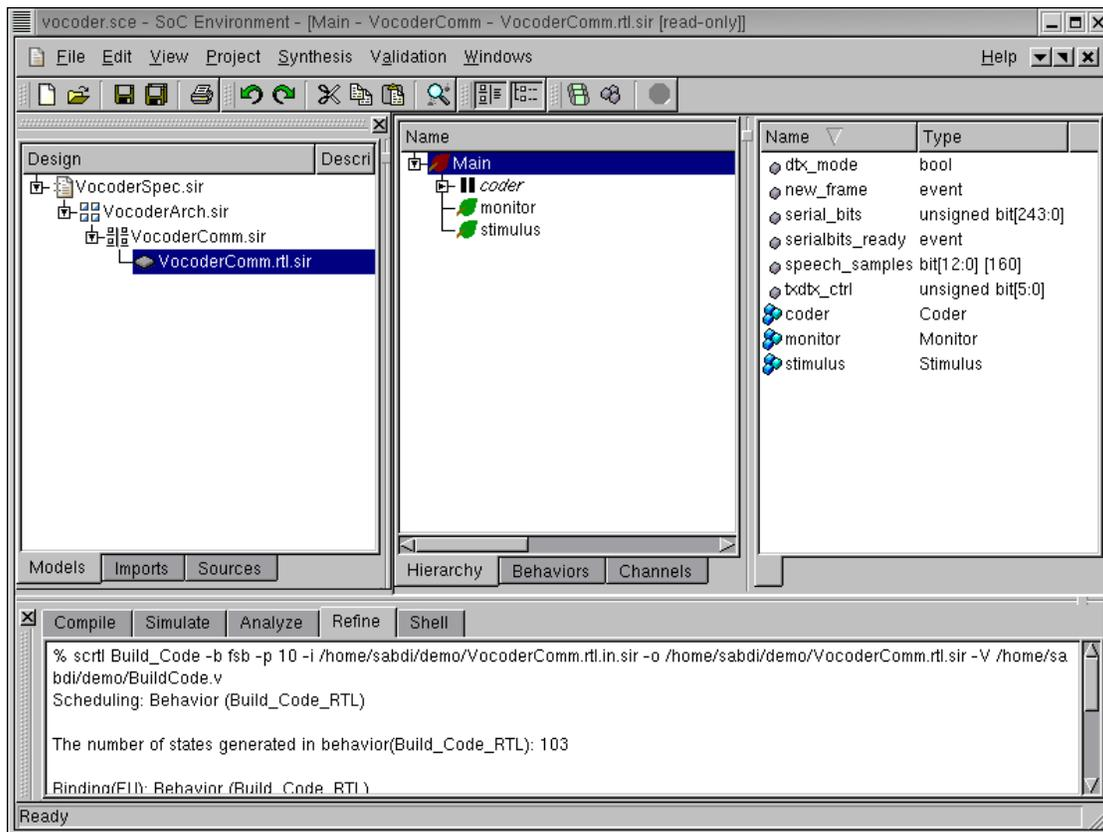
Note that RTL synthesis generates 103 states as seen on the logging window as the tool generated the RTL model for "BuildCode". Also note that a new model "VocoderComm.rtl.sir" is added in the Project manager window.
