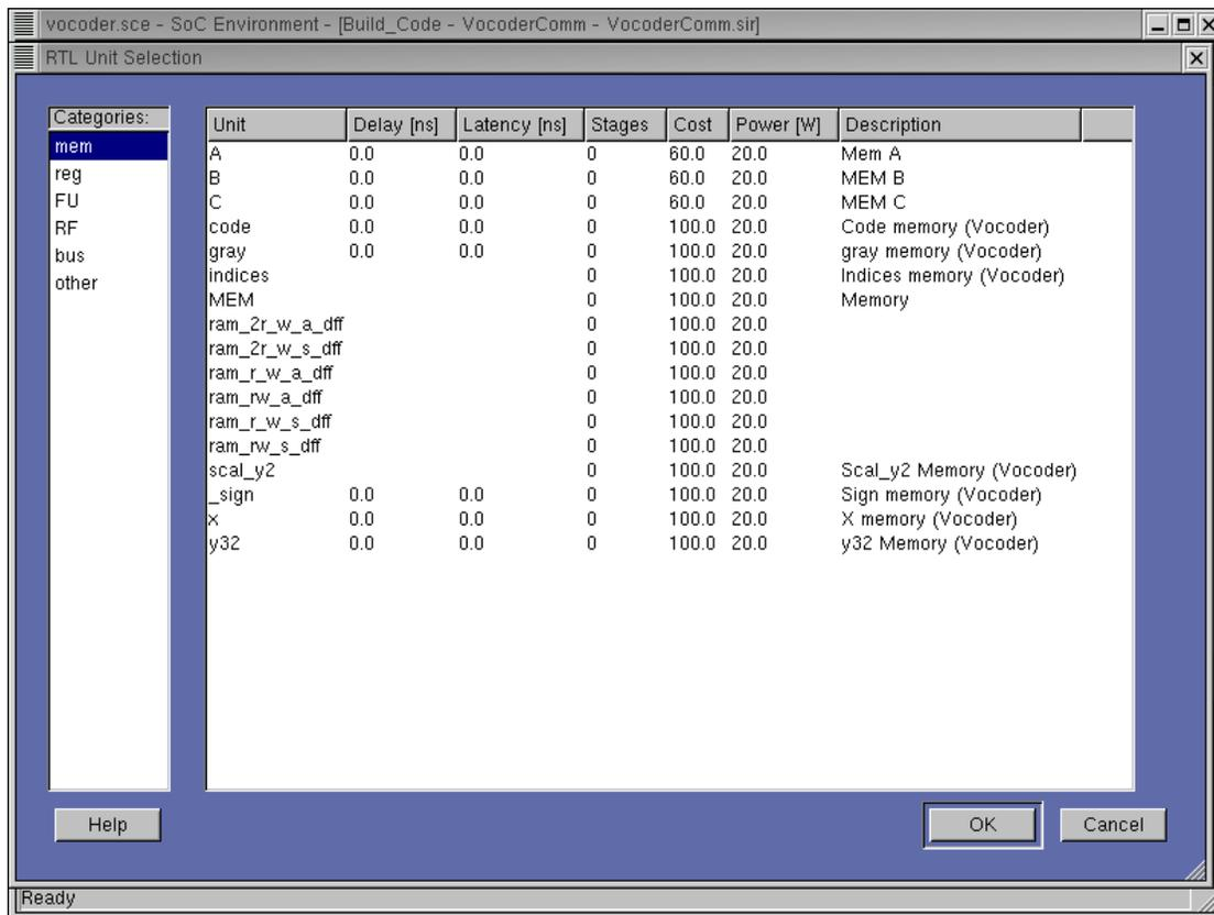
A new window pops up for RTL unit selection. There are various categories for the RTL units listed on the left-most column. Left click on "mem" to see the memory units and their properties.
