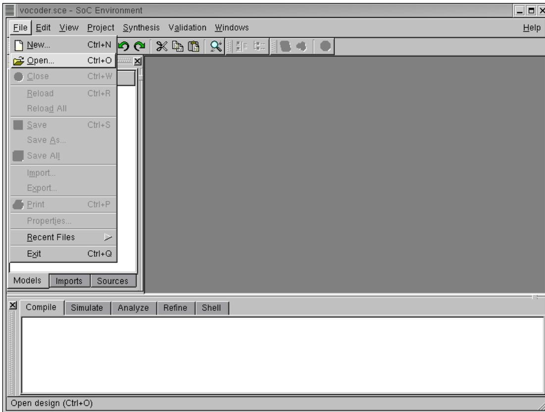
We start with the specification that was already captured as a model. We open this model to see if it meets the imposed constraints. Once the model is validated to be "golden", we will start refining it and adding implementation details to it. We open the specification model for the Vocoder example by selecting **File**→**Open** from the menu bar.
