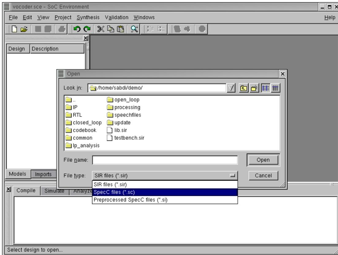
A file selection window pops up showing the SpecC internal representation (SIR) files. The internal representation files are a collection of data structures used by the tools in the environment. They uniquely identify a SpecC model. At this time however, the design is available only in its source form. We therefore need to start with the sources. Select "SpecC files (\*.sc)" to view the source files.
