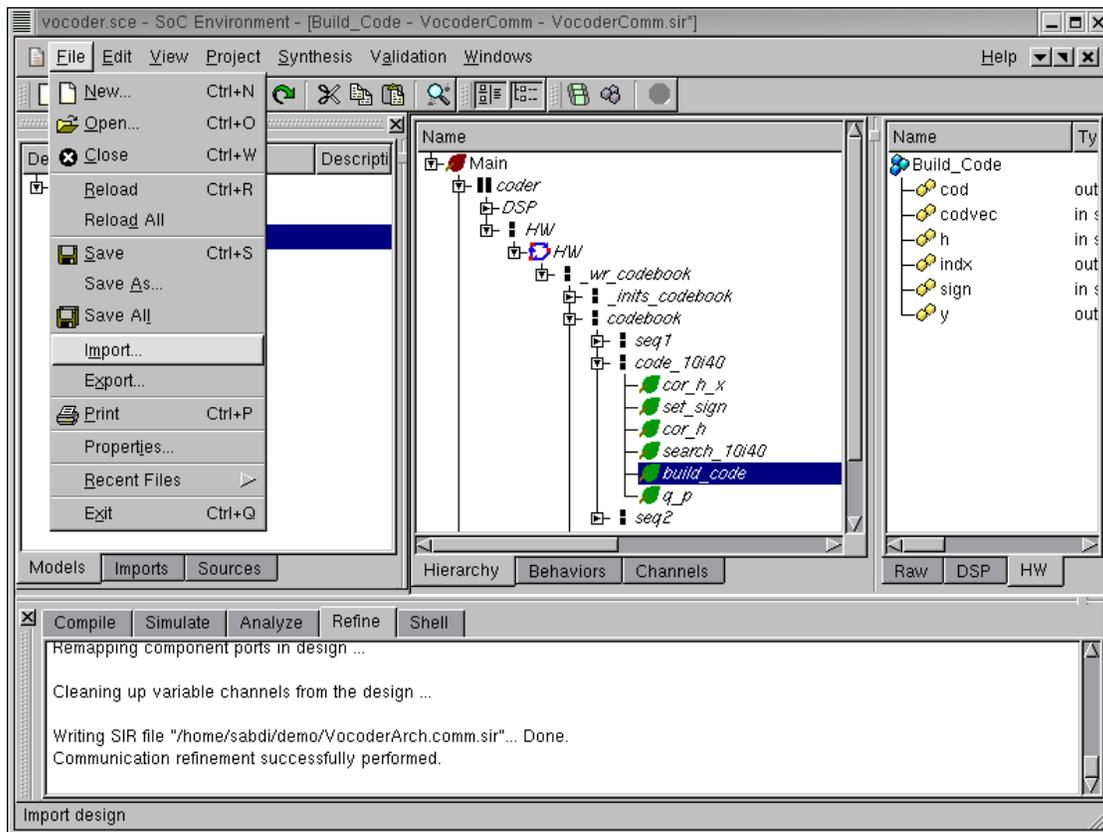
We now begin the RTL refinement process by importing the preallocated set of RTL units by selecting File→Import from the menu bar.
