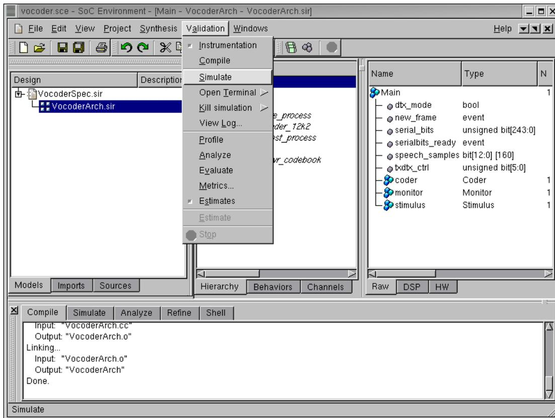
The messages in the logging window shows that the architecture model is compiled successfully without any syntax error. Now in order to verify that it is functionally equivalent to the specification model, we will simulate the compiled architecture model on the same set of speech data used in the specification validation. Go to **Validation** menu and select **Simulate** .
