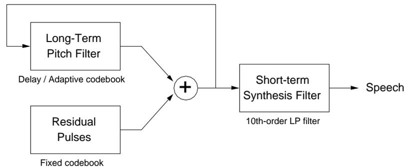
The example design used through out this tutorial is the GSM Vocoder system , which is employed worldwide for cellular phone networks. The figure shows the GSM Vocoder speech synthesis model. A sequence of pulses is combined with the output of a long term pitch filter. Together they model the buzz produced by the glottis and they build the excitation for the final speech synthesis filter, which in turn models the throat and the mouth as a system of lossless tubes.
