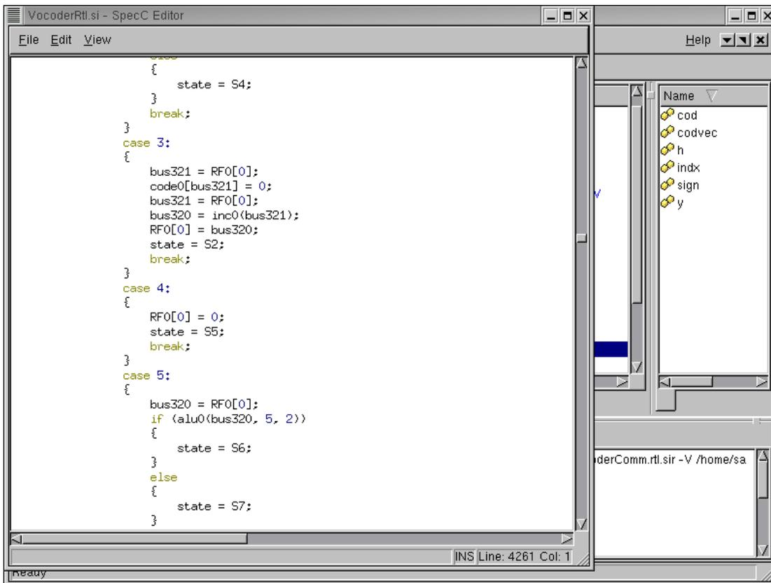
Further observations of the generated code show read/write operations on the register files. For instance RF0 is the register file written in the statement `bus321 = RF0[0]`; as shown in the code.
