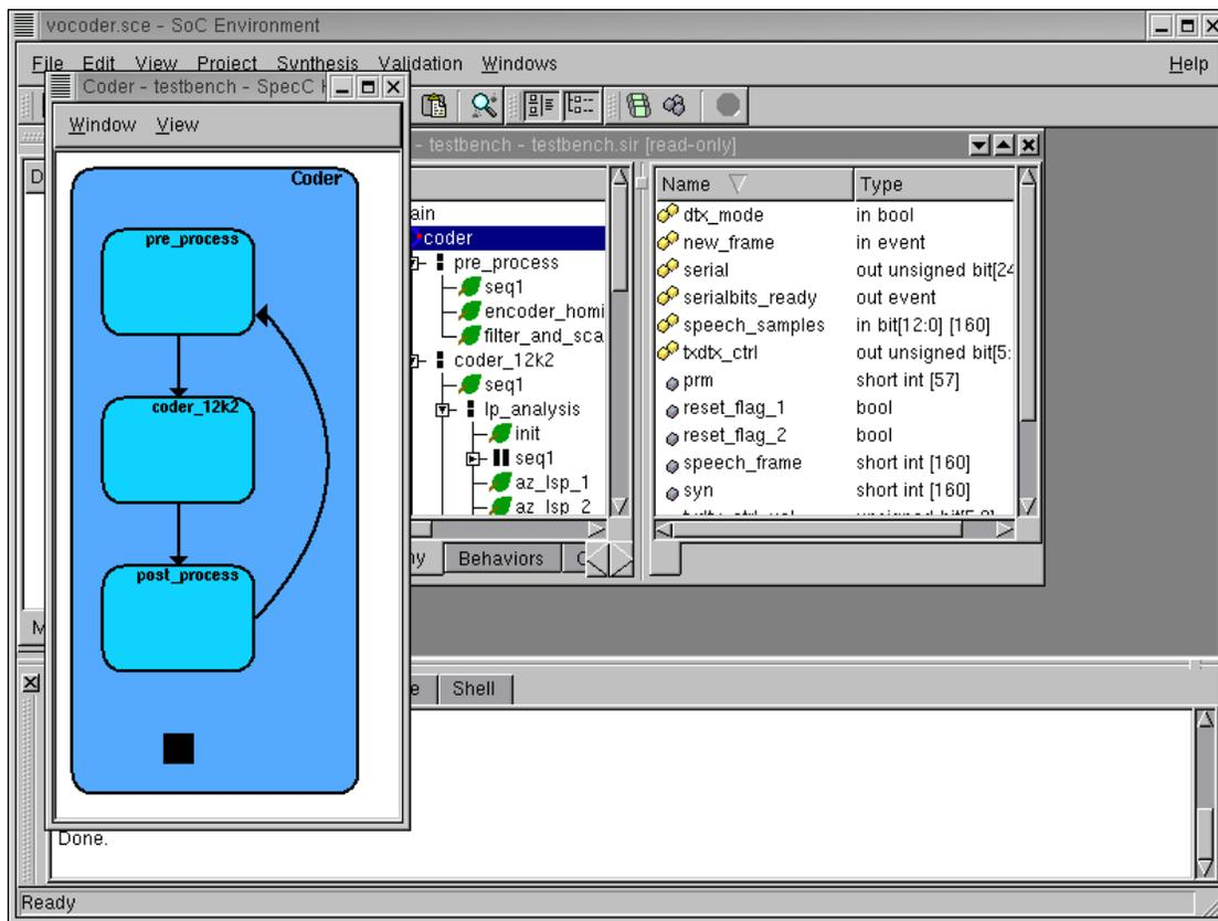
A new window pops up showing the Vocoder model in graphical form. As noted earlier, the specification is an FSM at the top level with three states of pre-processing, the bulk of the coder functionality itself and finally post-processing.
