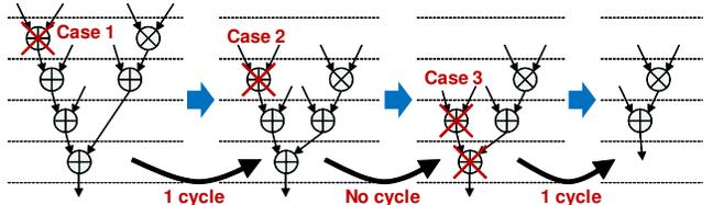
Fig. 3. Operation elimination and cycle reduction.
