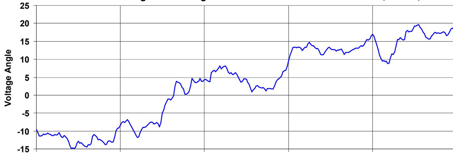
Wind MW generation is not presently available on ERCOT's public web site. However, by observing the voltage phase angle of West Texas with respect to U.T. Austin (i.e., central ERCOT), we believe that wind MW generation was low but on the rise at 5am when grid problems began, and that wind MW generation rose to moderate levels (approx. 10% of total generation) through the troubled 5am – 10am generation shortage period.
