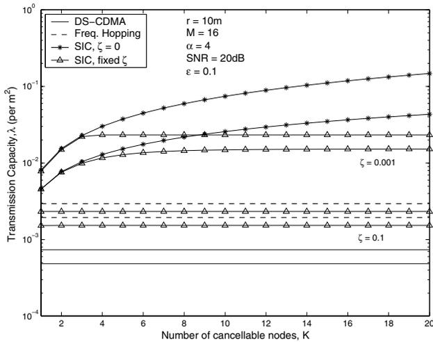
Fig. 4. Transmission capacity vs. number of cancellable users. Only a few interferers need to be cancelled to get most of the gain from SIC. This is because these closest interferers who cause most of the interference. In fact, unless the interference cancellation is extremely accurate, cancelling just one node gets most of the capacity of  $K = \infty$ . This outcome has favorable implications for receiver complexity and latency.
