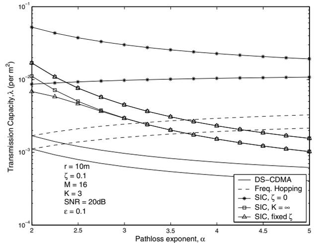
Fig. 3. Transmission capacity vs. path loss exponent. Direct sequence capacity reduces as the path loss becomes worse because much higher transmit power levels must be used, which further cripples the nearby nodes. In contrast, while frequency hopping nodes have the same problem, they only have a  $1/M$  chance of colliding with nearby nodes, and meanwhile, the farther nodes now cause less interference than before.
