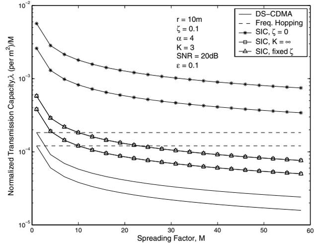
Fig. 2. Normalized transmission capacity vs. spreading factor. Since all DS-CDMA systems lose capacity as the spreading factor increases, the spreading factor should be chosen to be as small as possible while still allowing interference averaging.
