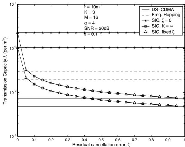
Fig. 5. Transmission capacity vs. residual cancellation error. Capacity degrades quite rapidly as interference cancellation error increases, with nearly 2 orders of magnitude difference between perfect cancellation and no cancellation ( $\zeta = 1$ ).
