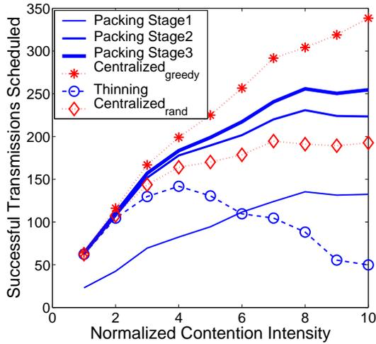
Figure 7: Performance of the Packing approach surpasses  $Centralized_{rand}$  when contention intensity at each stage is optimally chosen.
