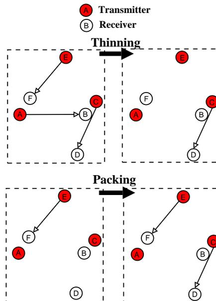
Figure 2: On the top, an example of thinning contenders with only one surviving transmission. On the bottom, an example of a packing of contenders with two surviving transmissions.
