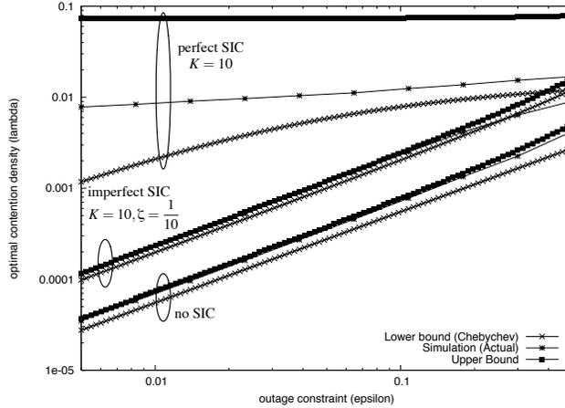
Figure 1: Optimal contention density  $\lambda^\epsilon$  versus the outage constraint  $\epsilon$  for the no SIC, imperfect SIC, and perfect SIC scenarios.
