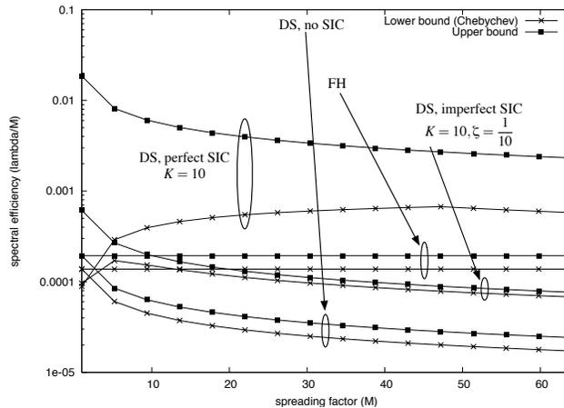
Figure 4: Spectral efficiency  $\lambda^\epsilon/M$  versus the spreading factor  $M$  for four scenarios: DS-CDMA with no SIC, DS-CDMA with imperfect SIC, DS-CDMA with perfect SIC, and FH-CDMA.
