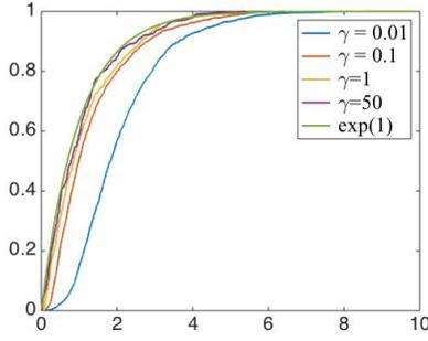
Fig. 4. CDF of interarrival of up-crossings for various thresholds
