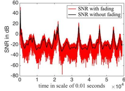
Fig. 5. SNR process in presence of fading with mean 1
