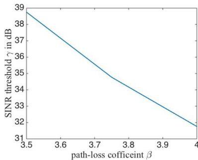
Fig. 7. Threshold above which the inter-arrival of up-crossing converge to exponential with parameter 1 for different path loss exponent
