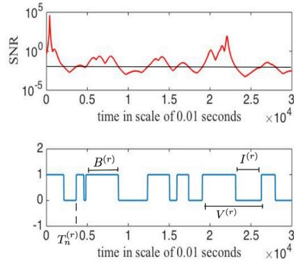
Fig. 2. Level Crossings of SNR process as On-Off Process
