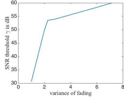
Fig. 6. Threshold above which the inter-arrival of up-crossing converge to exponential with parameter 1 for different variance of fading
