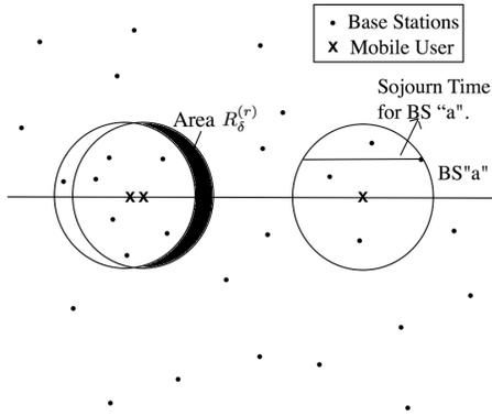
Fig. 1. Figure showing the disc around the mobile user with area  $R_\delta^{(r)}$  and the chord along which the node moves
