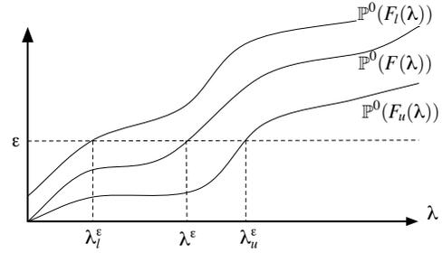
Fig. 2. Illustration of the technique to find lower and upper bounds on the contention density:  $\lambda_l^\epsilon \leq \lambda^\epsilon \leq \lambda_u^\epsilon$  through the use of necessary and sufficient events for outage.
