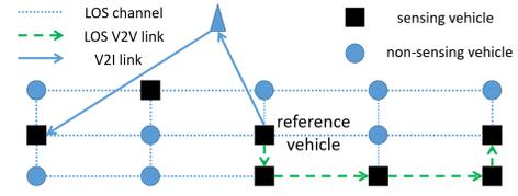
Fig. 8. Collaborative sensing of vehicles in a single lane using V2V + V2I, with V2V relay assistance from vehicles in the two neighboring lanes.
