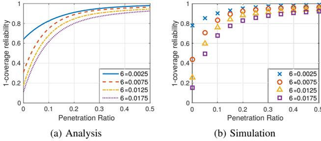
Fig. 6. 1-coverage reliability: (a) based on analytical approximation in Eq. 6, and (b) obtained by simulation of highway scenario.
