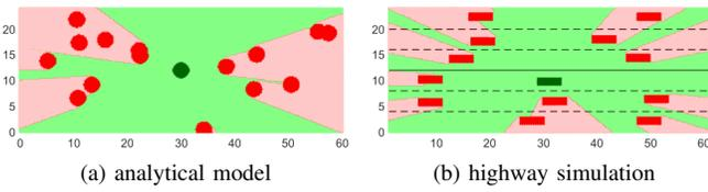
Fig. 4. Sensing of a typical vehicle in (a) analytical model and (b) highway simulation model. The green shapes are reference objects, the red shapes are obstructions, light green represents sensed region, light red indicates obstructed region.
