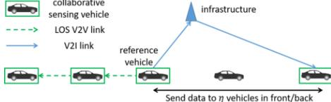
Fig. 7. Collaborative sensing of vehicles in a single lane with V2V + V2I network. Vehicle uses V2I to relay data when LOS V2V links are blocked.
