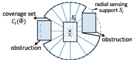
Fig. 3. Coverage set of sensor  $i$  in  $\tilde{\Phi}$ .
