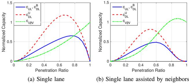
Fig. 9. How V2I capacity requirements, normalized by  $\lambda_v \cdot d \cdot \nu$ , scale with  $p_s$  in (a) single lane and (b) single lane assisted by vehicles in neighbor lanes.  $c_{UL}$  is uplink capacity,  $c_{DL}^B$  and  $c_{DL}^U$  are downlink capacity using broadcast and unicast.  $c_{V2V}$  is V2V throughput per sensing vehicle normalized by the V2V throughput at full penetration,  $p_s = 1$ .
