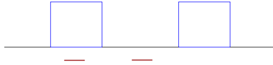
Figure 2.3: A periodic On/Off traffic constrained by e(t) = \min[pt, \rho t + \sigma] .
