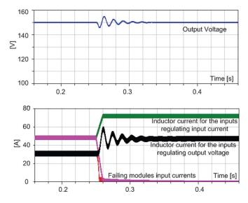
Fig. 11. Simulation showing the behavior of Configuration C with boost converters when failures occur at t = 0.25 s.
