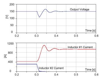
Fig. 10. Simulation showing the behavior of Configuration A with CSHB when a failure occurs at t = 0.3 s.
