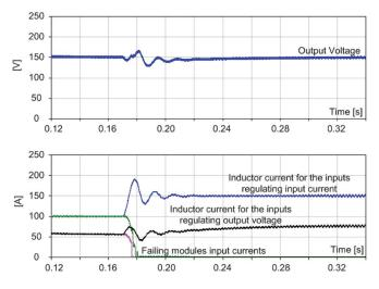
Fig. 12. Simulation showing the behavior of Configuration F with MI ISEPICs when failures occur at t = 0.17 s.
