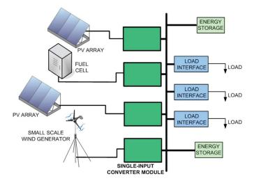
Fig. 1. Possible dc microgrid architecture with SICs.
