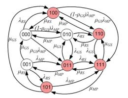
Fig. 16. Markov diagram for a conventional telecom energy system without considering the batteries.
