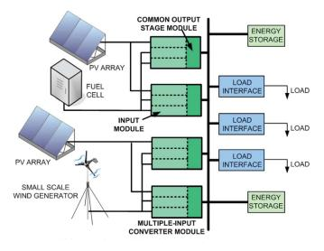
Fig. 2. Possible dc microgrid architecture with MICs.
