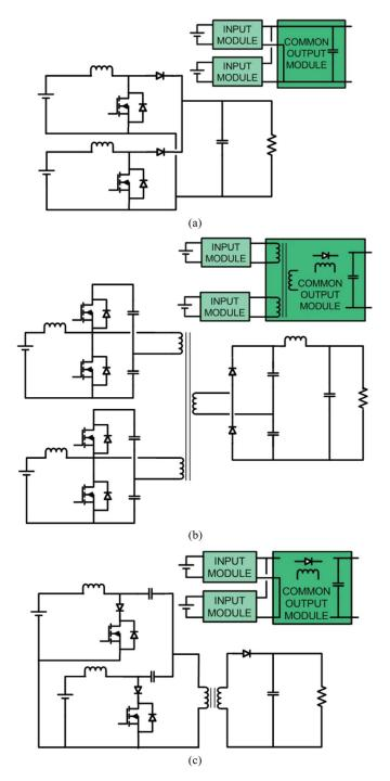
Fig. 3. Three possible MICs topologies. (a) Boost. (b) CSHB [40]. (c) ISEPIC.
