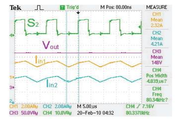
Fig. 14. Oscilloscope capture for a hardware prototype of a two-input ISEPIC. From top to bottom, the traces are: switching signal for the switch at the leg with the lowest input voltage (shown to provide an indication of the switching frequency), output voltage, input current at the leg with the highest voltage, and input current at the other leg.
