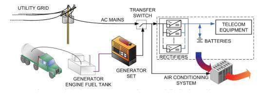
Fig. 15. Typical telecom energy system elements and distribution architecture.
