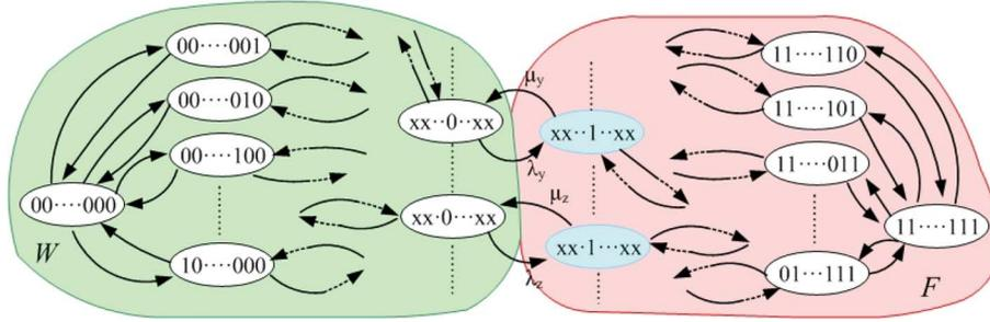
Fig. 5. General Markov representation of a micro-grid availability behavior with the minimal cut states indicated with a shaded interior.
