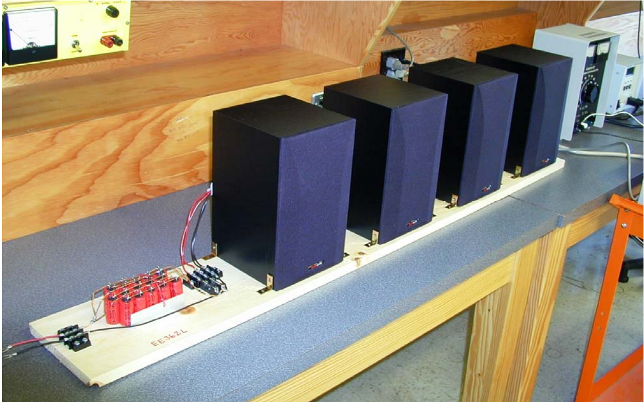
Four 8\Omega speakers in series present 32\Omega to the inverter
