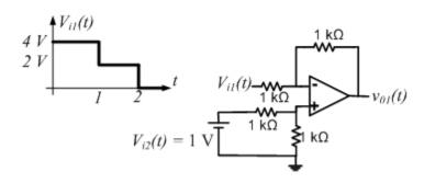
Using  $v_{0l}(t)$  as your input voltage for the next circuit, sketch the output voltage  $v_0(t)$ considering that at the initial time t=0,  $v_0(t=0)=0$
